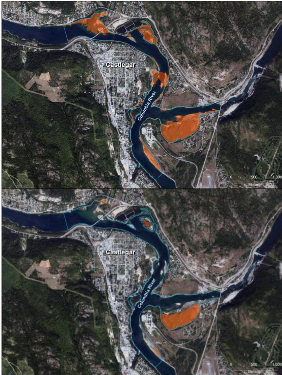
Figure 5-8: The available shoreline areas between the river and the high-water mark (orange areas) at the minimum (417.88 m in Feb. 2016, top panel) and maximum (422.14 m in Dec. 2013, bottom panel) water elevations present in the study area between November 1 and February 28 of survey years. Water elevation was measured from the CNN gauge at Norns Creek (source BC Hydro). The bounds of the area for this analysis are outlined in blue
