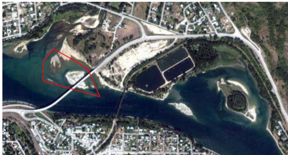
Figure 6-2: Potential area (red polygon) where physical works could be implemented to enhance existing sandbars to be resistant to inundation by increasing height to 422 m or higher. In this photo Waldie Island is visible to the right of the figure, with Breakwater Island occurring directly south of the Castlegar Sewage Lagoons.
