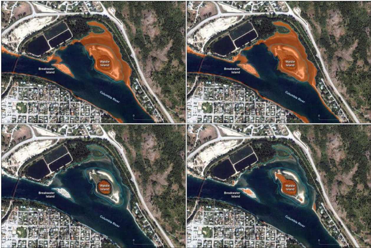
Figure 5-9: The available shoreline areas between the river and high-water mark (orange areas) at the minimum and maximum water elevations present around Waldie Island between Nov. 1 and Feb. 28 of survey years. Top Left=Feb. 2014 (418.42 m), Bottom Left=Dec. 2013 (422.14 m), Top Right=Feb. 2016 (417.88 m), Bottom Right=Jan. 2016 (420.39 m). Water elevation was measured from the CNN gauge at Norns Creek (source BC Hydro). The bounds of the area for this analysis are outlined in blue
