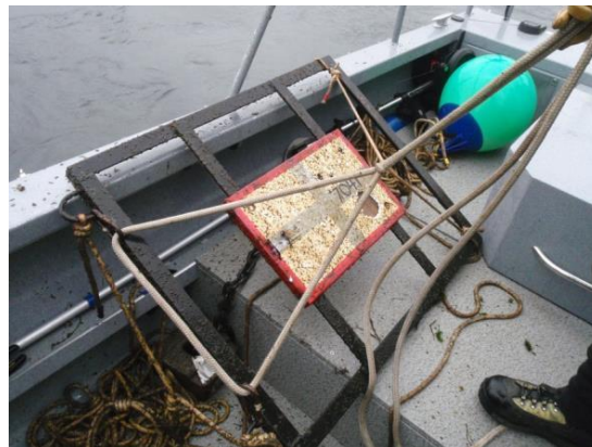
Figure 2-4: The Chandelier Deployment Method
