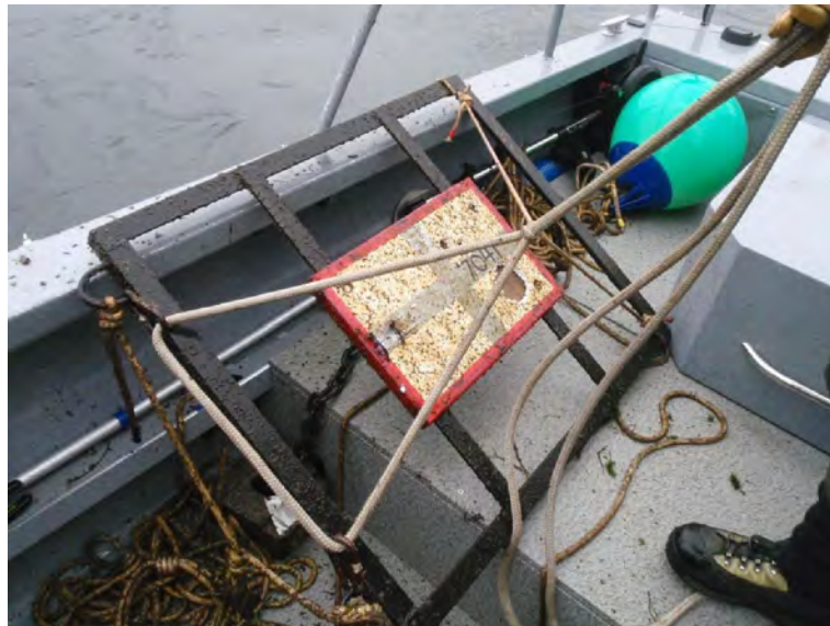
Figure 2-5: The Chandelier Deployment Method
