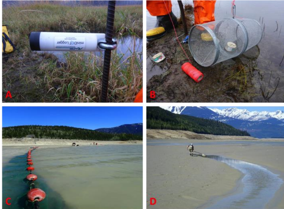
Photo 4. A. MiniDOT data logger deployed in a high elevation pool in fall 2017. B. Minnow trap baited with canned cat food. C. Beach seine net deployed in a large low elevation isolated pool. D. Dip netting was an effective method for catching fish in shallow isolated pools.
