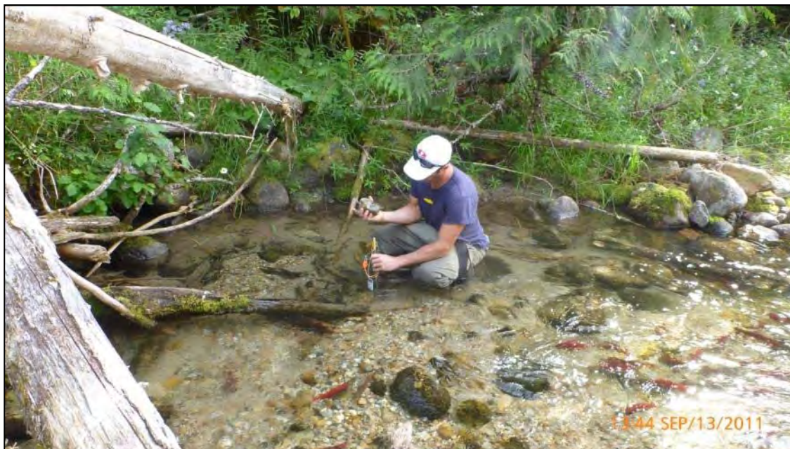
Photo Plate 3: Looking towards HOBO data logger installation along the left bank of Taite Creek in a side channel using a combination of rebar and galvanized wire. The previously installed Taite Creek data logger was lost during freshet, with the logger separating from the epoxy.
