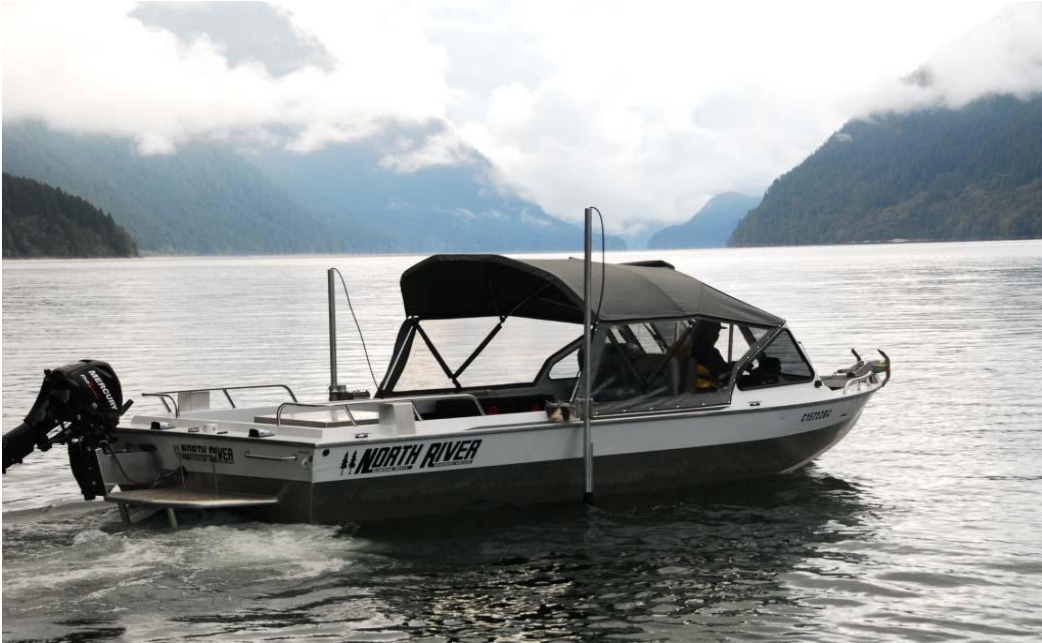
Photo 1. Jet boat equipped for tracking with vertically adjustable hydrophone holders mounted on either side.
