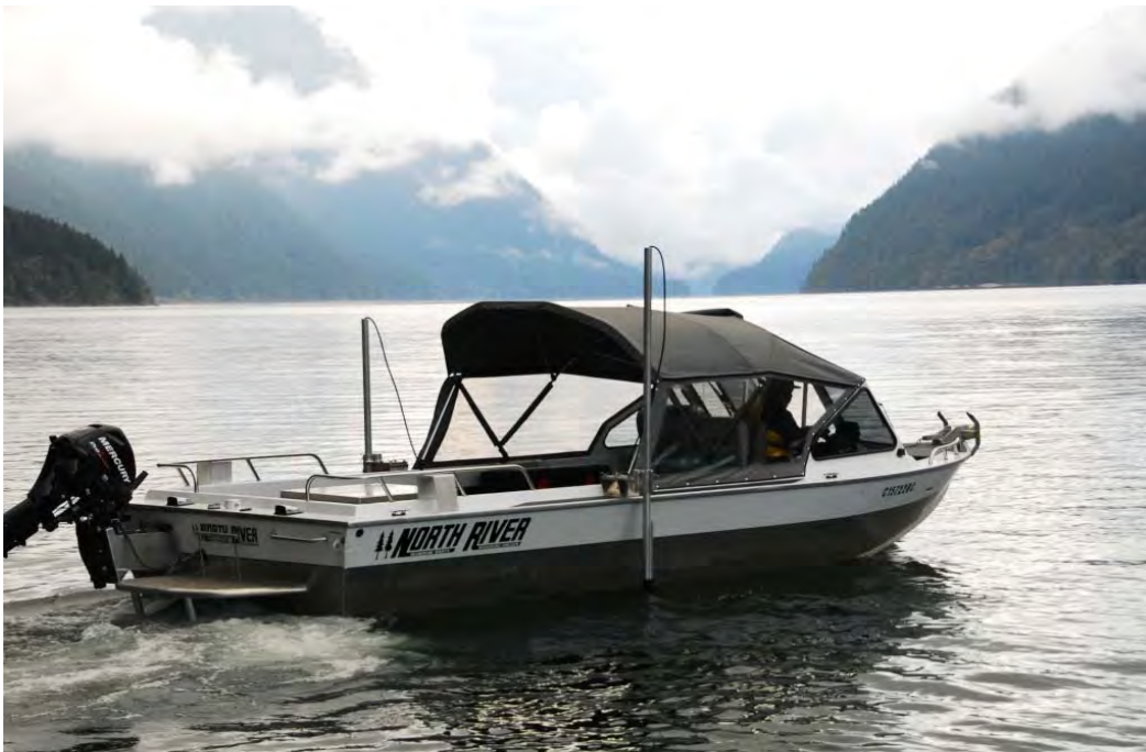
Photo 3. Jet boat equipped for tracking with vertically adjustable hydrophone holders mounted on either side.
