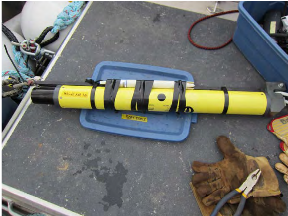
Acoustic release (yellow) with attached SBE56 (white) in back of the boat, 29 Aug 2013
