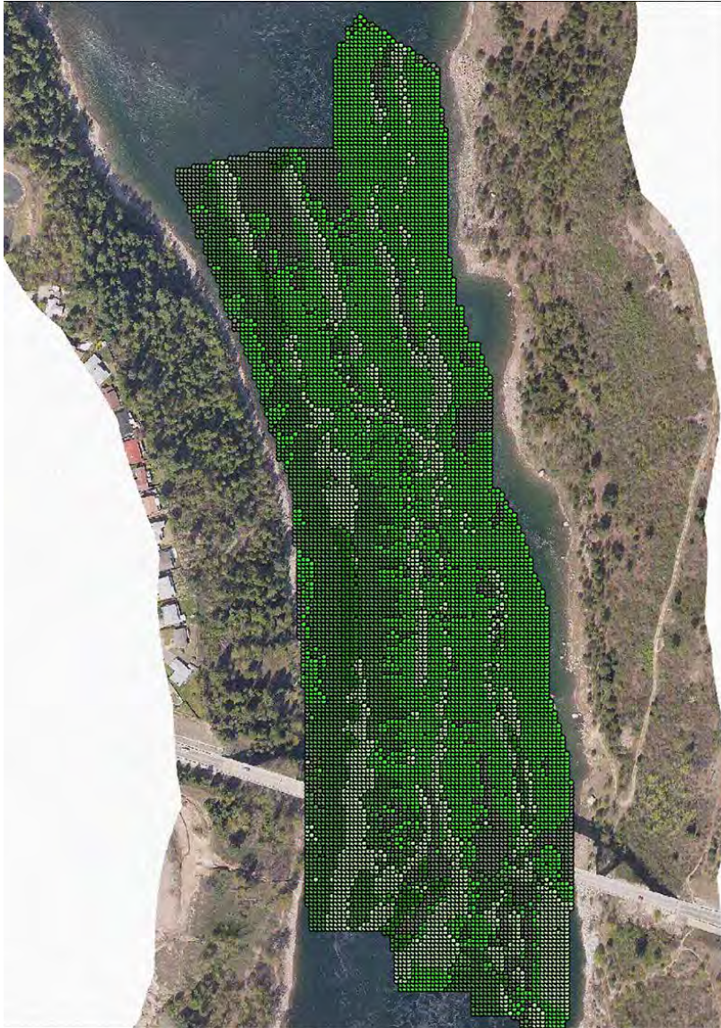
Figure 20. An example of acoustic backscatter data classified into substrate types (Colour patterns) that was collected in the lower Columbia River using a side scan sonar. The validation of substrate types is ongoing.
