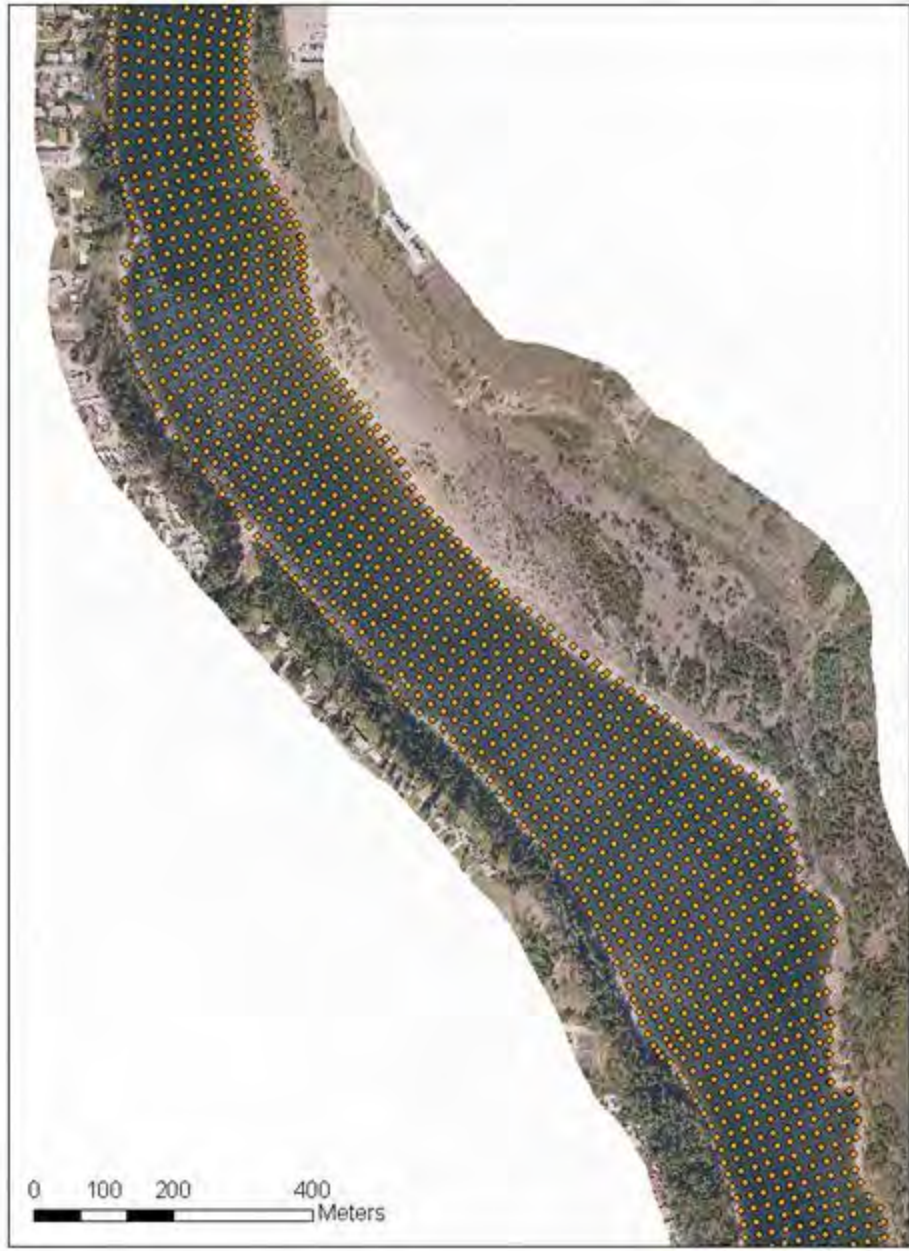
Figure 4. An example of transects generated to collect physical habitat data in the lower Columbia River, British Columbia. Transects were run perpendicular to the flow and points were spaced at 20 m intervals moving downstream.
