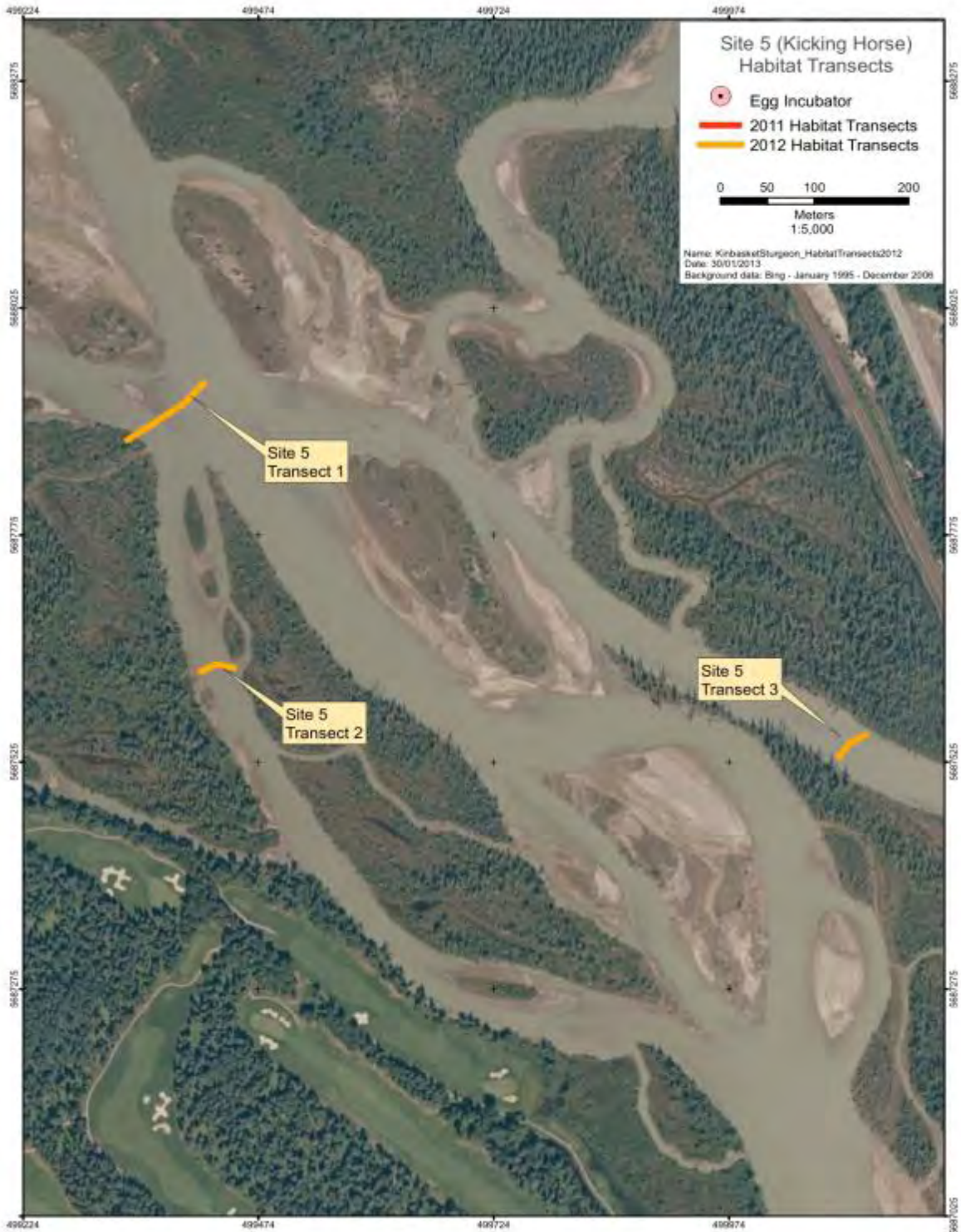
Figure B4 Columbia River Habitat Assessment Site 5 immediately downstream of Kicking Horse River. The overview shows transect locations in order from upstream (transect 3) to downstream (transect 1). Within each transect, measurements of depth, velocity, substrate and turbidity were taken at five locations: right bank (RB), right midbank (RM), thalweg, left midbank (LM) and left bank (LB).
