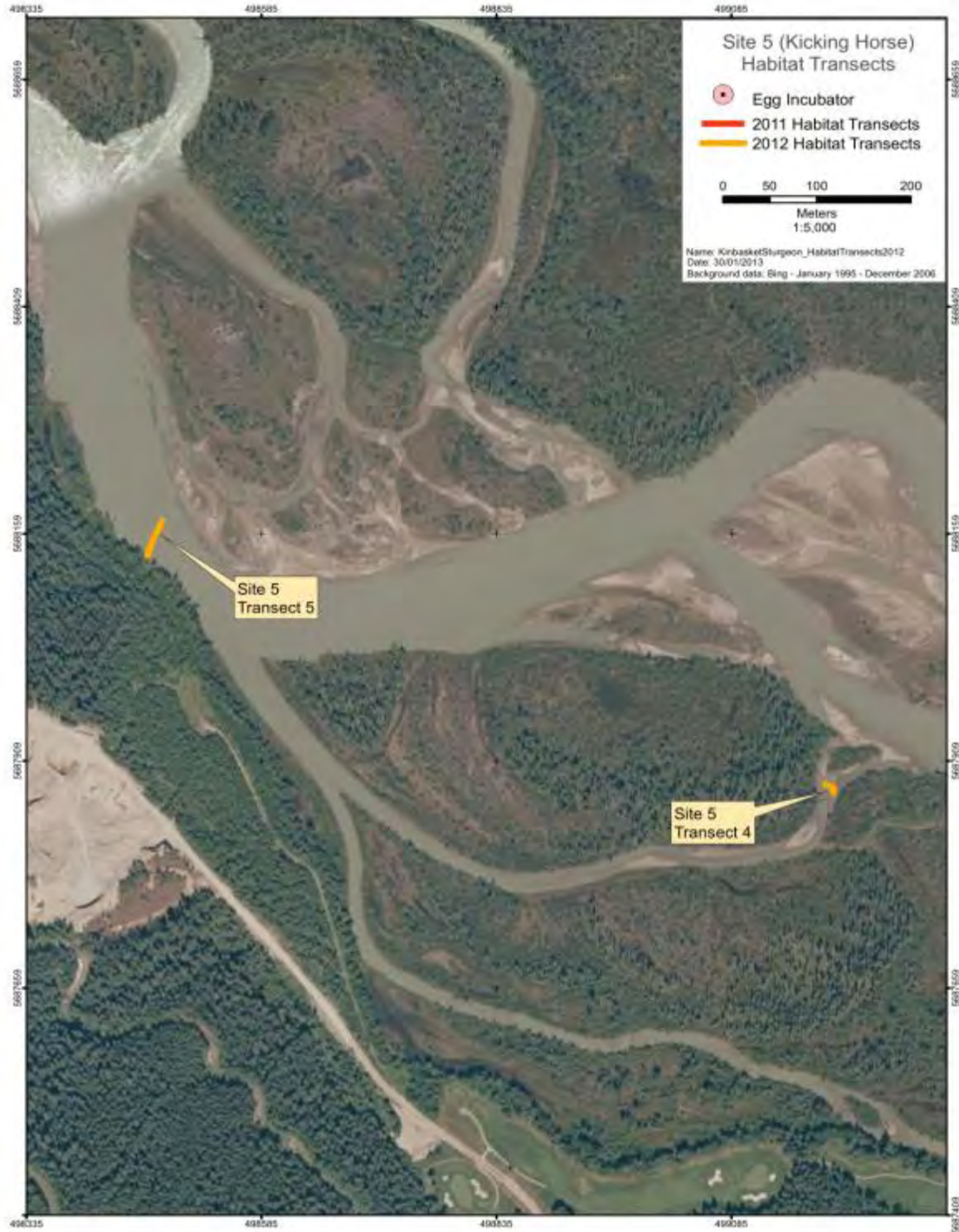
Figure B4 cont. Columbia River Habitat Assessment Site 5 immediately downstream of Kicking Horse River. The overview shows transect locations in order from upstream (transect 4) to downstream (transect 5). Within each transect measurements of depth, velocity, substrate and turbidity were taken at five locations: right bank (RB), right midbank (RM), thalweg, left midbank (LM) and left bank (LB).
