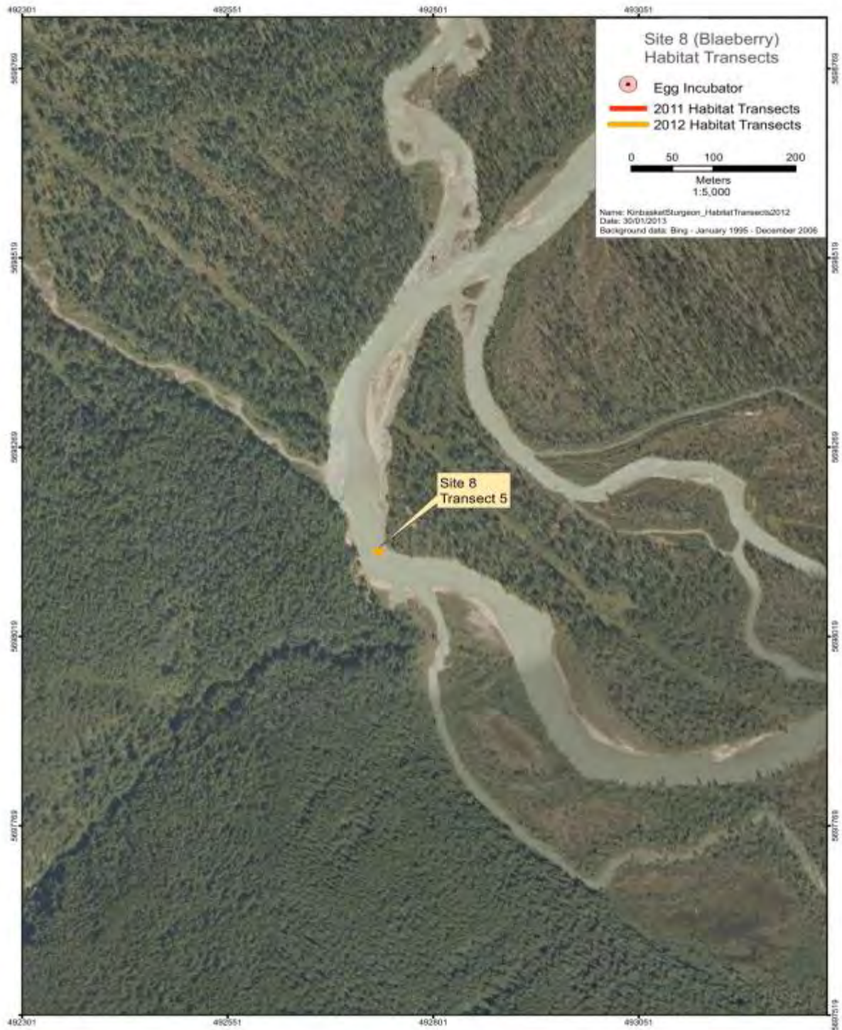
Figure B7 con't Columbia River Habitat Assessment Site 8 at Blaeberry BC. Transect 5 is the most downstream measurement at this site. Within each transect, measurements of depth, velocity, substrate and turbidity were taken at five locations: right bank (RB), right midbank (RM), thalweg, left midbank (LM) and left bank (LB).
