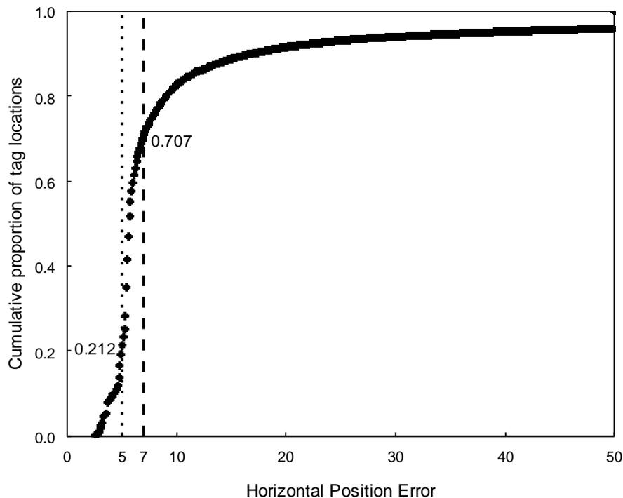
Figure 4: Cumulative proportion of tag positions in relation to HPE (Horizontal Position Error). The cumulative proportions of tag positions at HPE = 5 and HPE = 7 are provided on the graph.
