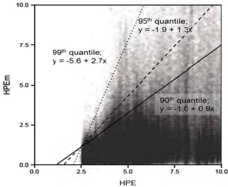
Figure 3: HPEm as a function of HPE for all synchronization and reference tags; points represent individual estimated positioning errors. A transparency value of 0.01 was imposed, hence at least 100 points must overlap to create a solid black point. The lines and equations of three regressions (90th, 95th, and 99th quantiles) are plotted (solid, dashed, and dotted lines, respectively).
