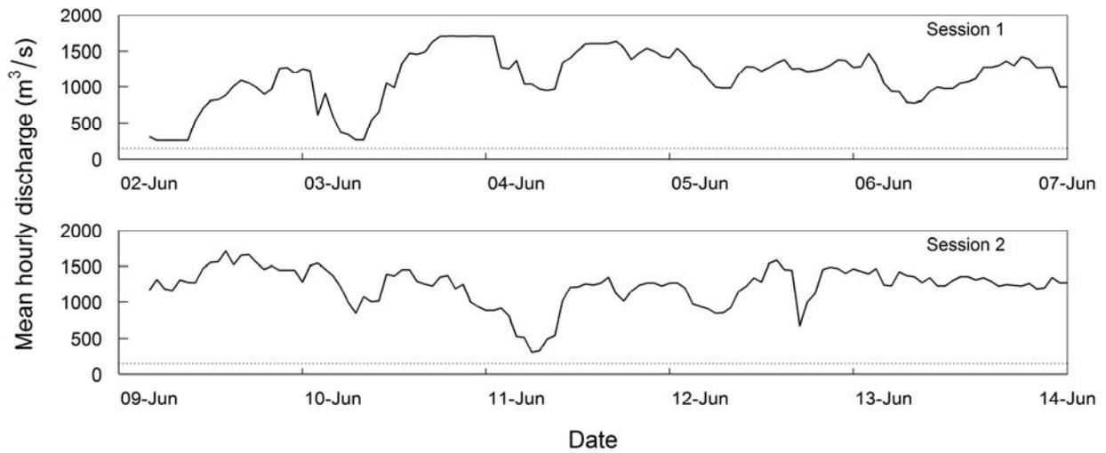
Figure C2 Mean hourly discharge (m<sup>3</sup>/s) for the Columbia River at Revelstoke Dam by sample session, June 2 to June 14, 2015. The dotted line denotes the 142 m<sup>3</sup>/s minimum flow release.
