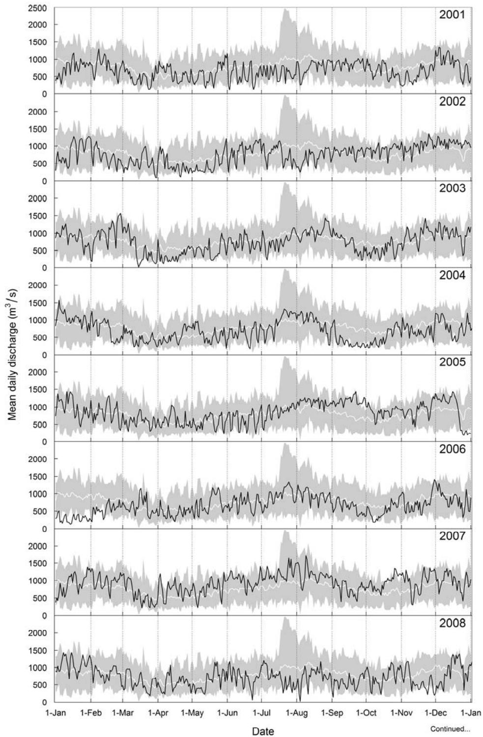
Figure C1 Mean daily discharge (m<sup>3</sup>/s) for the Columbia River at Revelstoke Dam, 2001 to 2015. The shaded area represents minimum and maximum mean daily discharge values recorded at Revelstoke Dam during other study years (between 2001 and 2015). The white line represents average mean daily discharge values over the same time period.
