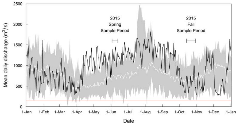
**Figure 2: Mean daily discharge ( $\text{m}^3/\text{s}$ ) for the Columbia River at Revelstoke Dam, 2015. The shaded area represents minimum and maximum mean daily discharge values recorded at the dam from 2001 to 2014. The white line represents average mean daily discharge values over that same time period. The red line represents the minimum flow release of  $142 \text{ m}^3/\text{s}$ .**
