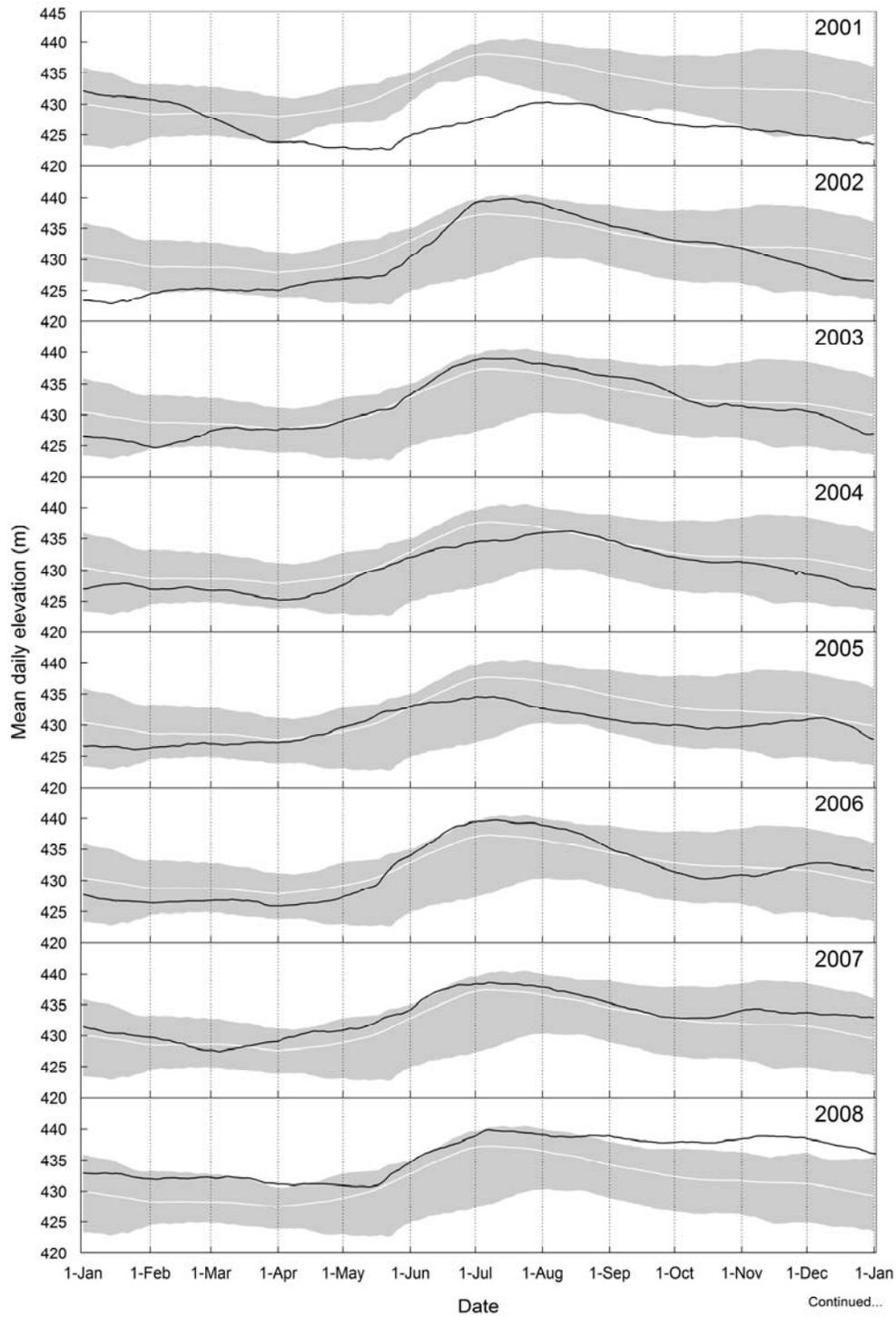
Figure C4 Mean daily water level elevation (in metres above sea level) for the Columbia River at Nakusp, 2001 to 2015. The shaded area represents minimum and maximum mean daily water elevations recorded at Nakusp during other study years (between 2001 and 2015). The white line represents average mean daily water elevation over the same time period.
