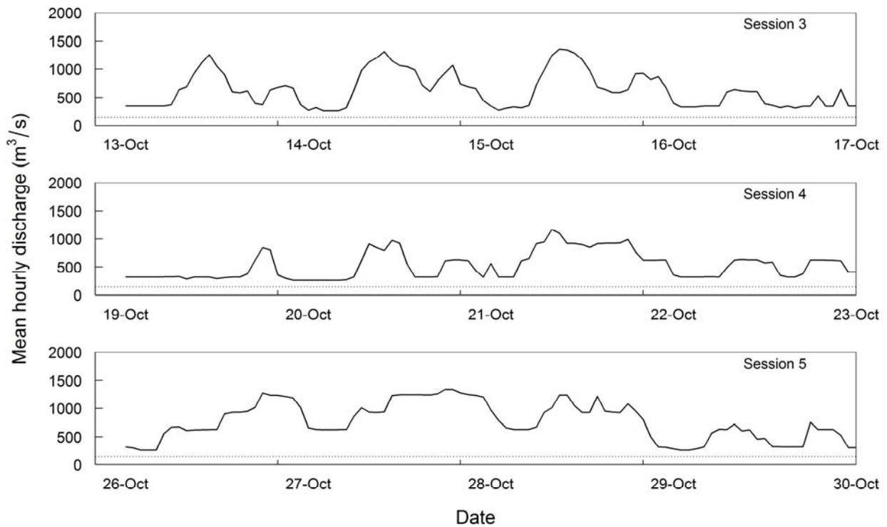
Figure C3 Mean hourly discharge (m<sup>3</sup>/s) for the Columbia River at Revelstoke Dam by sample session, October 13 to October 30, 2015. The dotted line denotes the 142 m<sup>3</sup>/s minimum flow release.
