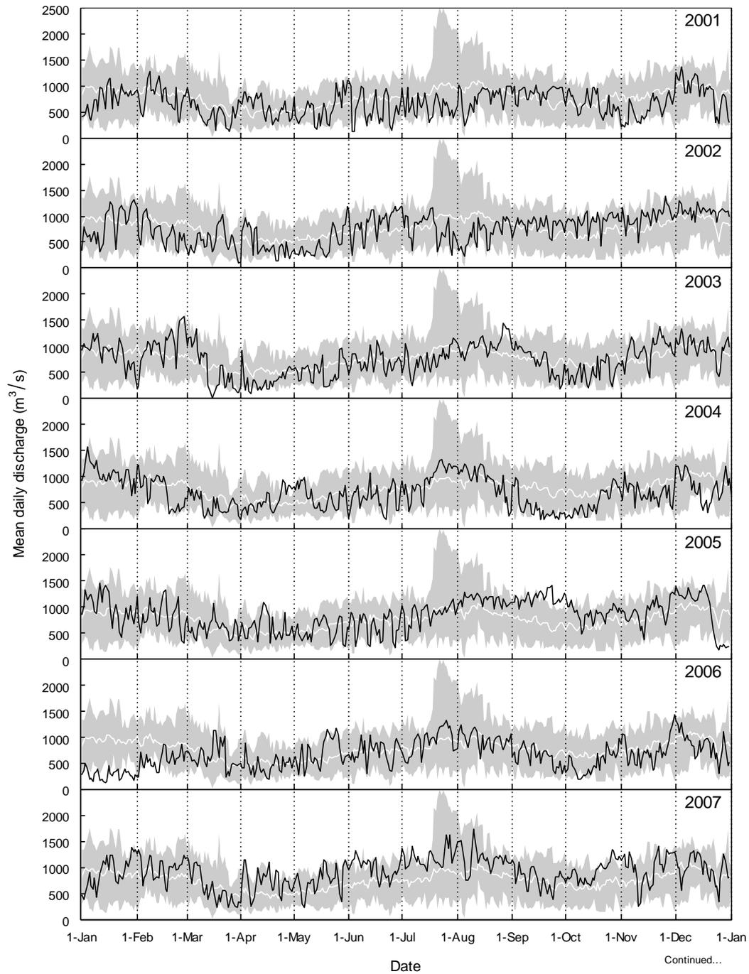
Figure C1 Mean daily discharge (m<sup>3</sup>/s) for the Columbia River at Revelstoke Dam, 2001 to 2013. The shaded area represents minimum and maximum mean daily discharge values recorded at Revelstoke Dam during other study years (between 2001 and 2013). The white line represents average mean daily discharge values over the same time period.
