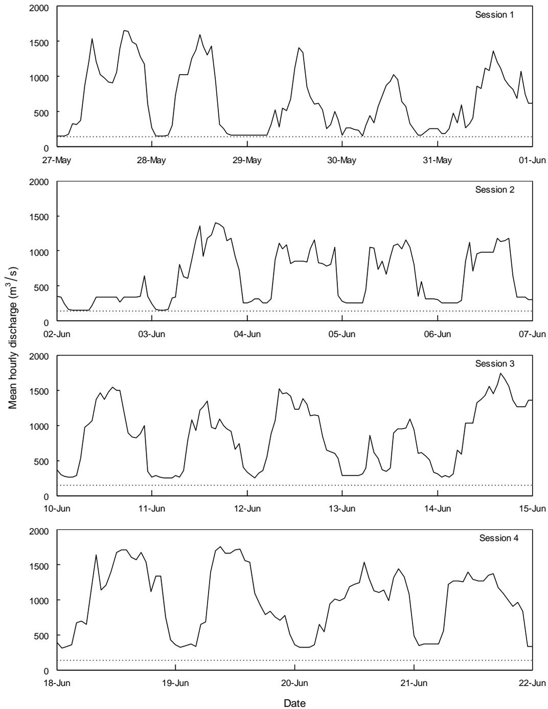
Figure C2 Mean hourly discharge (m<sup>3</sup>/s) for the Columbia River at Revelstoke Dam by sample session, May 27 to June 20, 2013. The dotted line denotes the 142 m<sup>3</sup>/s minimum flow release.
