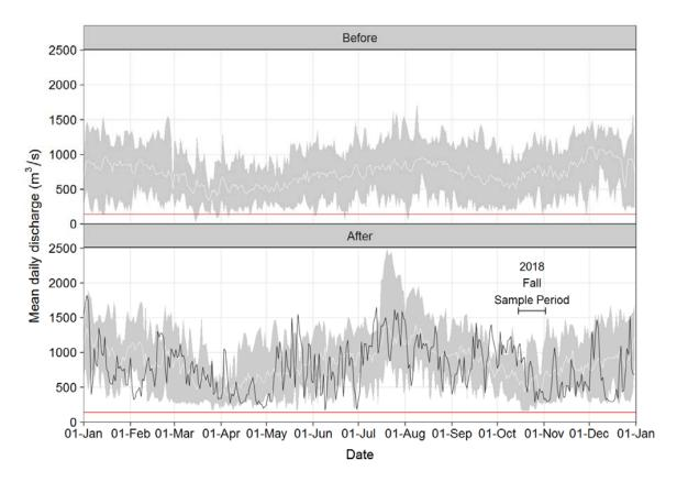
Figure 2: Mean daily discharge (m³/s) for the Columbia River at Revelstoke Dam in 2018 (black line) compared to historical discharge before and after the flow regime change. The shaded area represents minimum and maximum mean daily discharge values recorded at the dam from before (2001 to 2010) and after (2011 to 2017) the flow regime change. The white line represents average mean daily discharge values over those time periods. The red line represents the minimum flow release of 142 m³/s.
