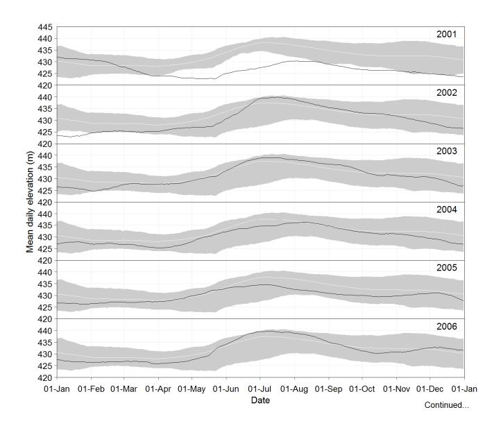
Figure C3 Mean daily water level elevation (in metres above sea level) for the Columbia River at Nakusp, 2001 to 2018. The shaded area represents minimum and maximum mean daily water elevations recorded at Nakusp during other study years (between 2001 and 2018). The white line represents average mean daily water elevation over the same time period.
