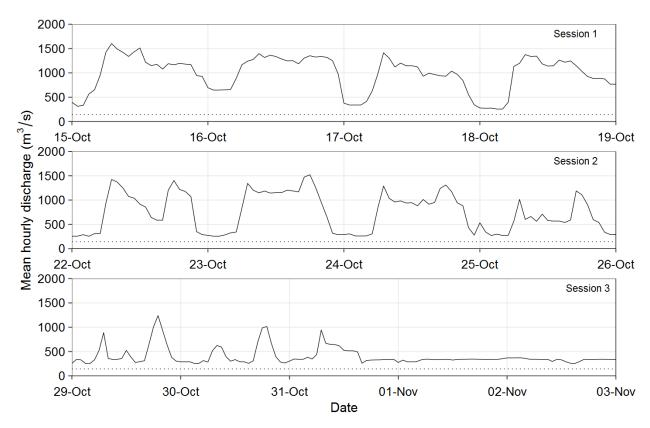
Figure C2 Mean hourly discharge (m³/s) for the Columbia River at Revelstoke Dam by sample session, 15 October to 2 November 2018. The dotted line denotes the 142 m³/s minimum flow release.
