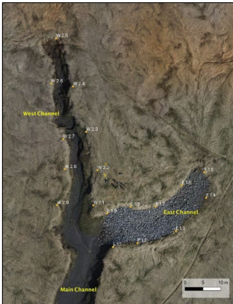
Figure 4-2: Image showing the arrangement of survey pins around the perimeter of the erosion channels. Thalweg measurements were taken between adjacent pins. Image date April 26, 2019
