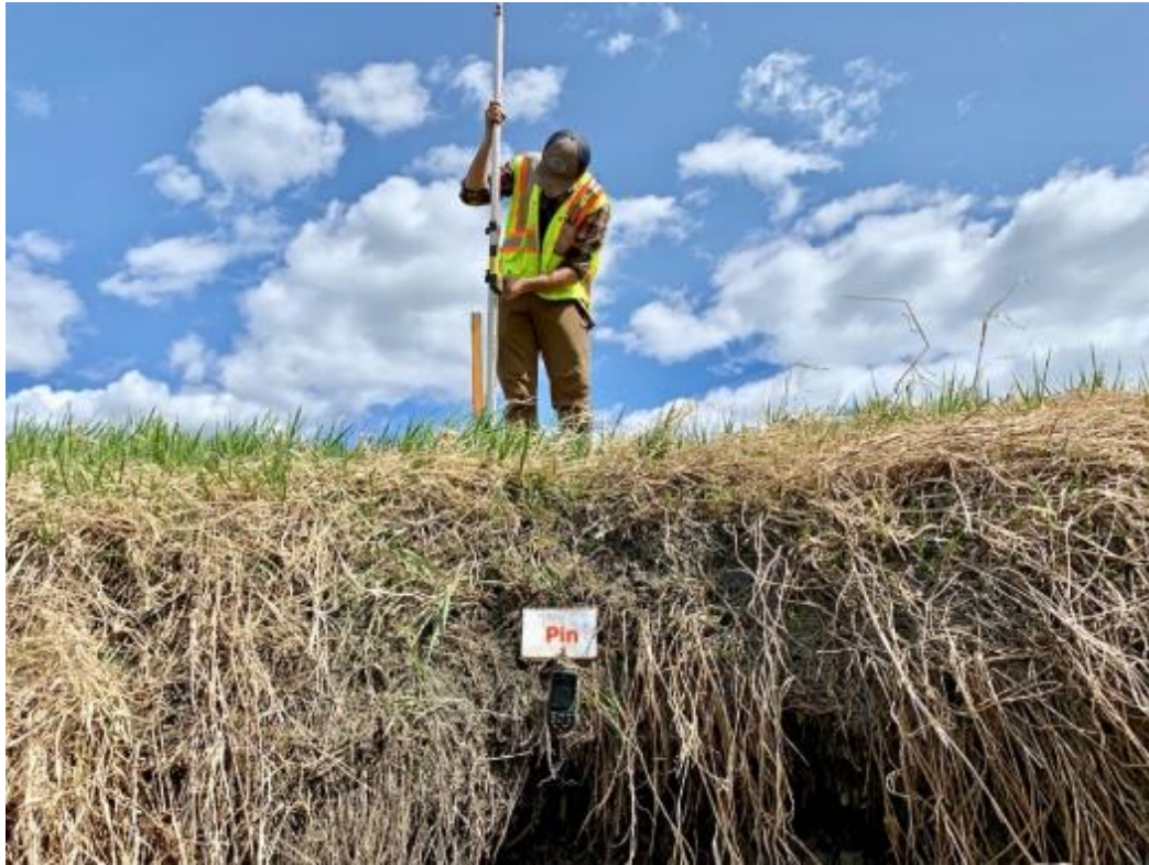
Figure 5-5: Photo of pin 2-4 located in the now overhanging (cantilevered) sod of the undercut bank of the west erosion channel. May 9, 2019.
