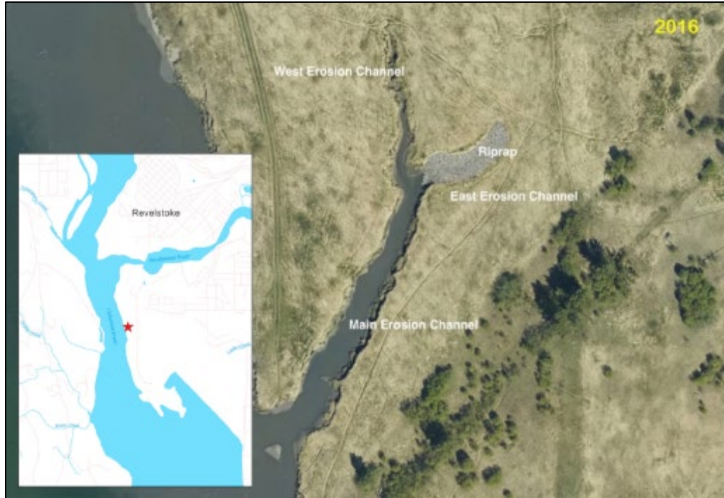
Figure 2-1: Aerial image of the WPW-6A “Y shaped” erosion channel. Scale 1:500. Inset show the location of the channel south of Revelstoke, BC. Image date May 2016.
