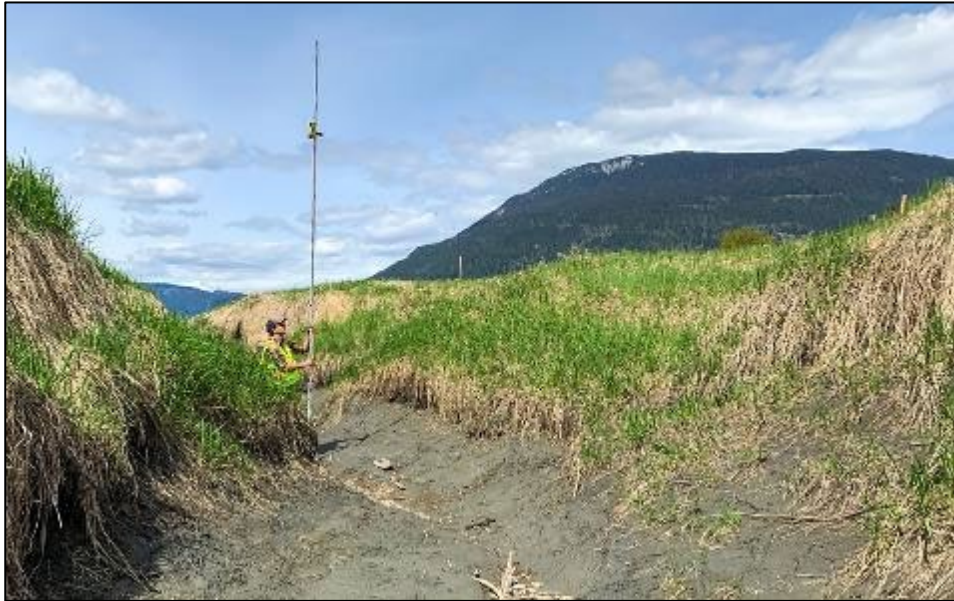
Figure 4-5: Image showing thalweg measurement being taken by ONG technician Addison Fosbery between erosion pins in the west erosion channel at WPW Site 6-A on May 9, 2019.
