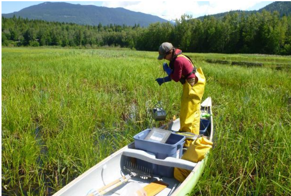
Figure 4-4: ONA researcher deploying the Ponar benthic sampler at Airport Marsh
