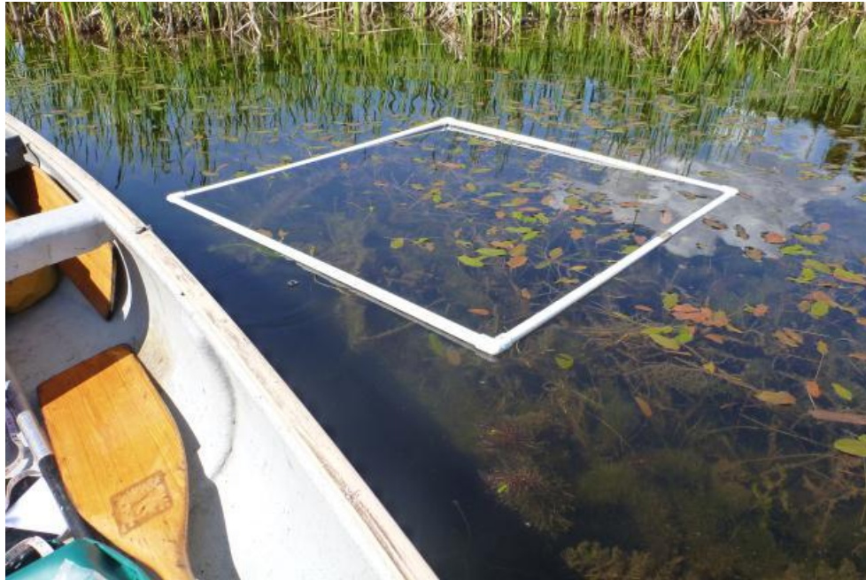
Figure 4-2: Buoyant, 1 m x 1 m PVC quadrat frame used for sampling floating aquatic vegetation
