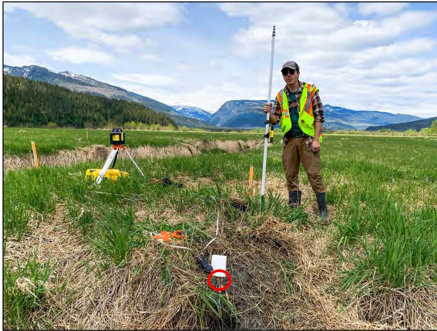
**Figure 4-2:** Image showing survey measurements taken at WPW Site 6-A. Environmental technician Addison Fosbery (Okanagan Nation Alliance) is standing above an erosion pin located in the red circle. Behind is the survey stake located 122 cm behind the erosion pin.
