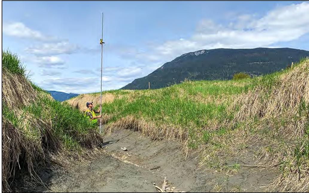
**Figure 4-4:** Image showing thalweg measurement being taken by Addison Fosbery between erosion pins in the west erosion channel at WPW Site 6-A. Note the bank failure that has occurred in the foreground (right hand bank).
