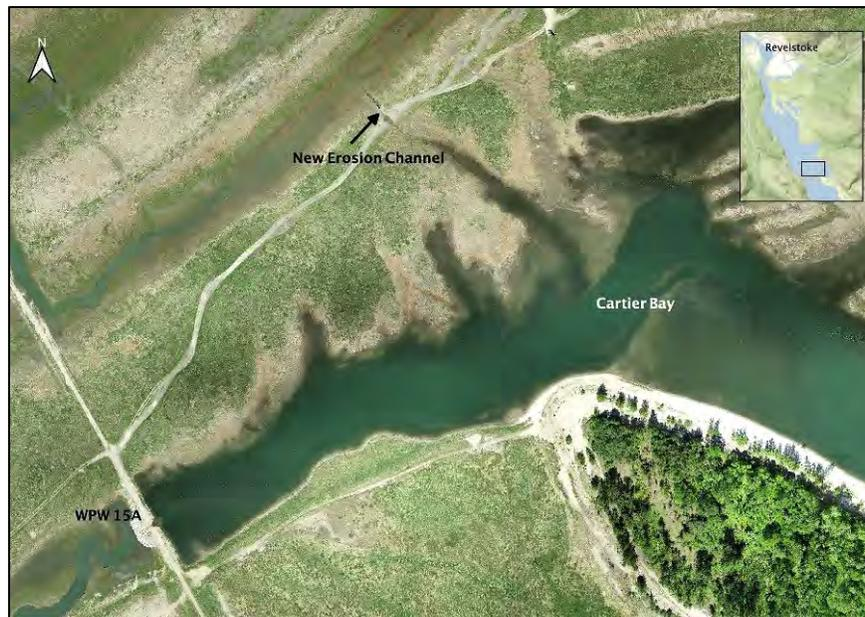
Figure 5-7. Location of recent erosion channel and head-cut (indicated by yellow arrow) caused by overflow from the west compartment of Cartier Bay wetland.
