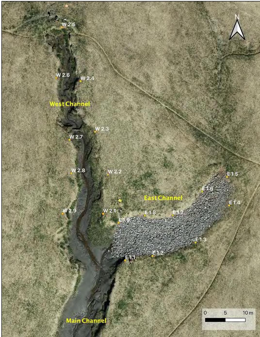
Figure 4-1: Image showing the arrangement of survey pins around the perimeter of the erosion channels. Thalweg measurements were taken between adjacent pins. Image date April 26, 2019
