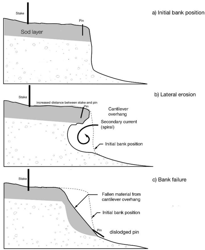
**Figure 4-3:** Diagram showing the process of bank undercutting, cantilevering, soil movement, bank failure, and slumping in relation to survey pin measurements. Adapted from Johnson and Stypula 1993.
