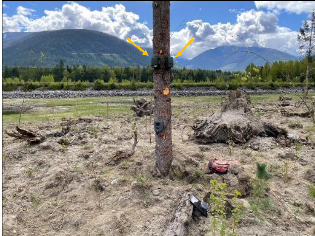
Figure 6-1. An acoustic (left) and ultrasonic (right) ARU attached to a snag above a wildlife camera in the WPW area in 2021. Credit: D. Adama.
