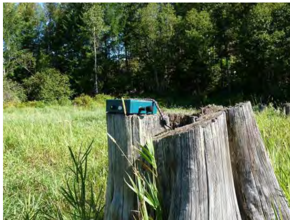
Figure 4-1: Example of a typical Song Meter SM2BAT unit set-up on an elevated feature with the microphone aimed in the direction of the desired habitat
