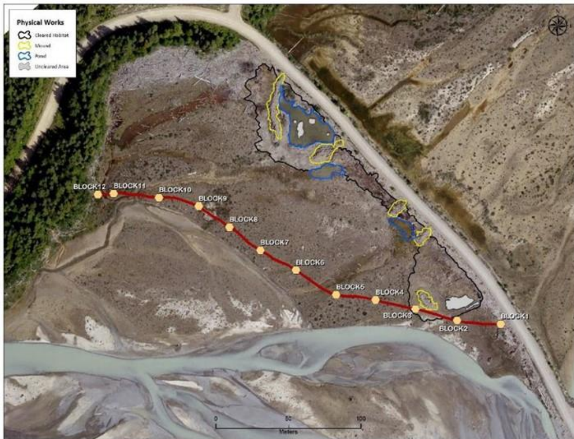
Figure 6-24: The Bush Causeway North site showing physical works treatment mounds (yellow polygons), cleared ponds (blue polygons), and log boom installation (red line). Photo: Hawkes 2017.
