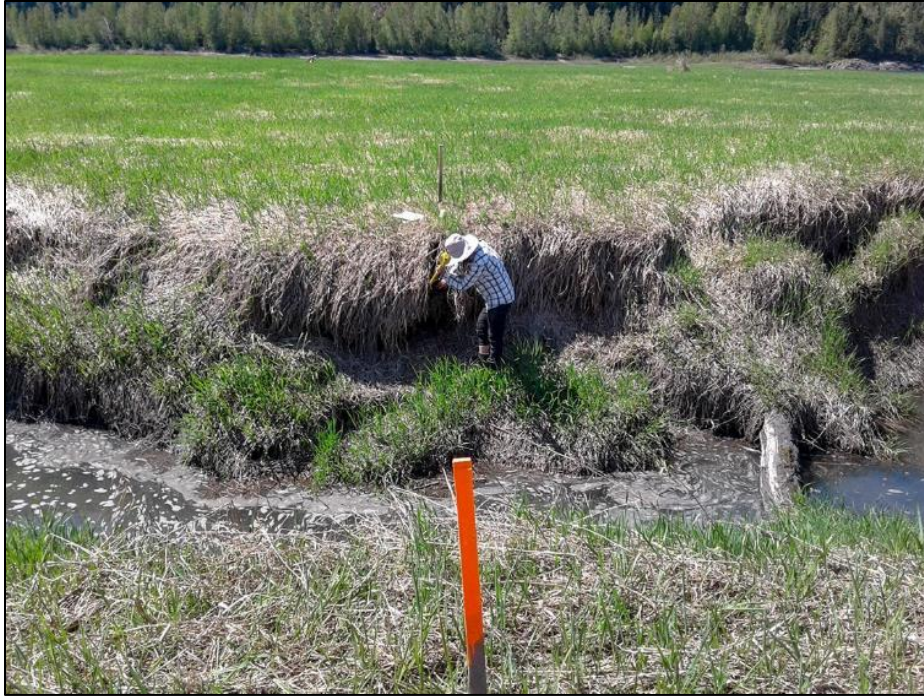
Figure 5-4: Autumn Solomon (ONA) searching for erosion pin 2.7 on an undercut bank in the west erosion channel at WPW-6A, May 2018.
