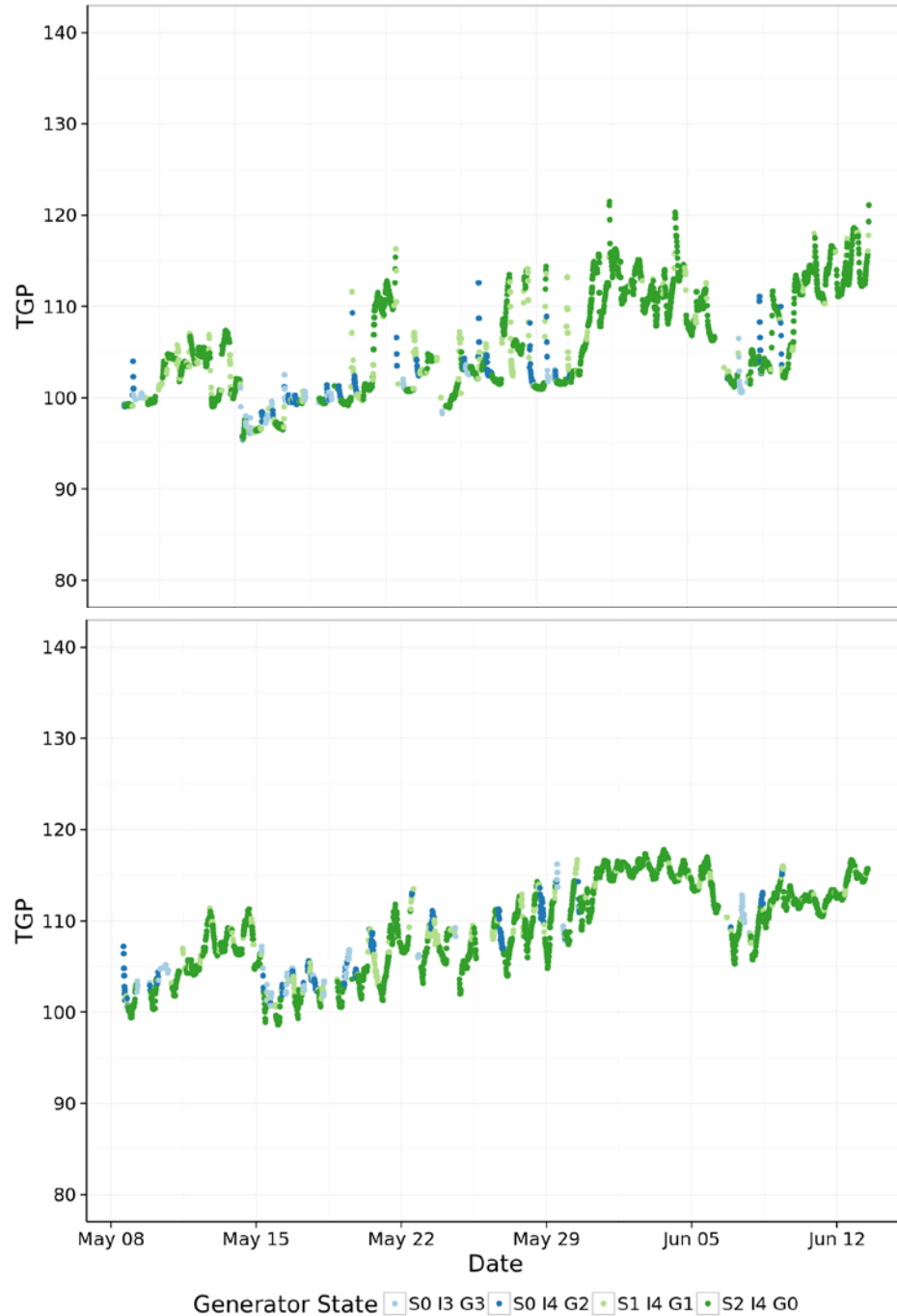
Figure 12. TGP generated by the combination of operating states over time from May 9 - June 13, 2017 measured at 0.2 km (Stn0) distance (top panel) and at 3.5 km (Stn1) distance (bottom panel) from MD.
