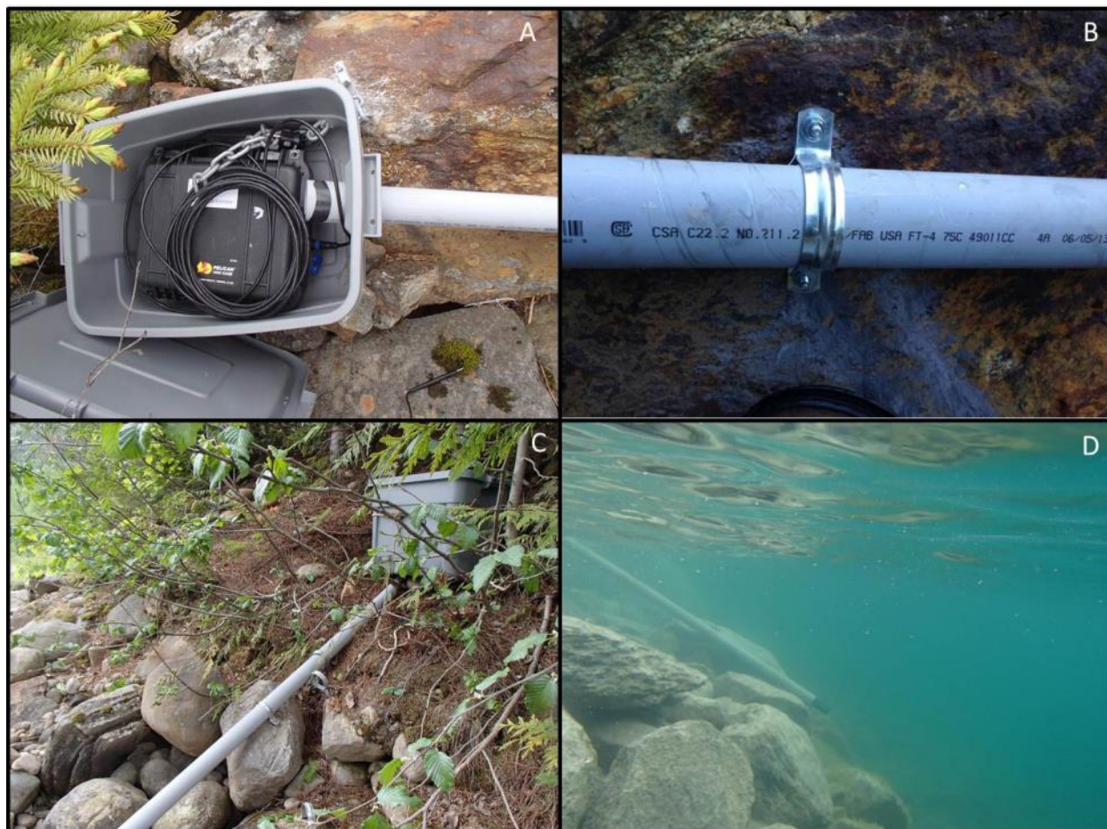
Figure 4. (A) TGP meter set-up at a station including pelican case, tote, chain and lock, and probe entering standpipe. (B) Example of an anchor for the standpipe. (C) Completed Station set-up with standpipe extending from TGP meter into the water. (D) Sonde extending 10 cm out of standpipe under water.
