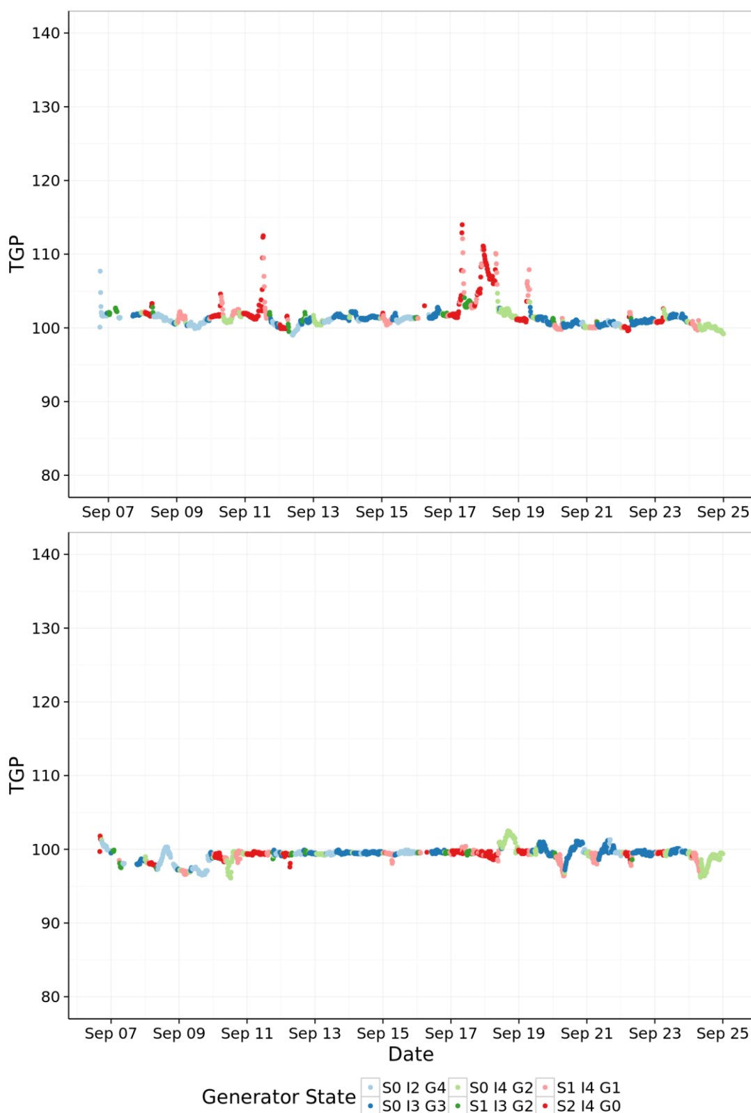
Figure 21. TGP generated by the combination of operating states over time from September 6 to 25, 2016 measured at 0.2 km distance (top panel) and 3.5 km distance (bottom panel) from MD.
