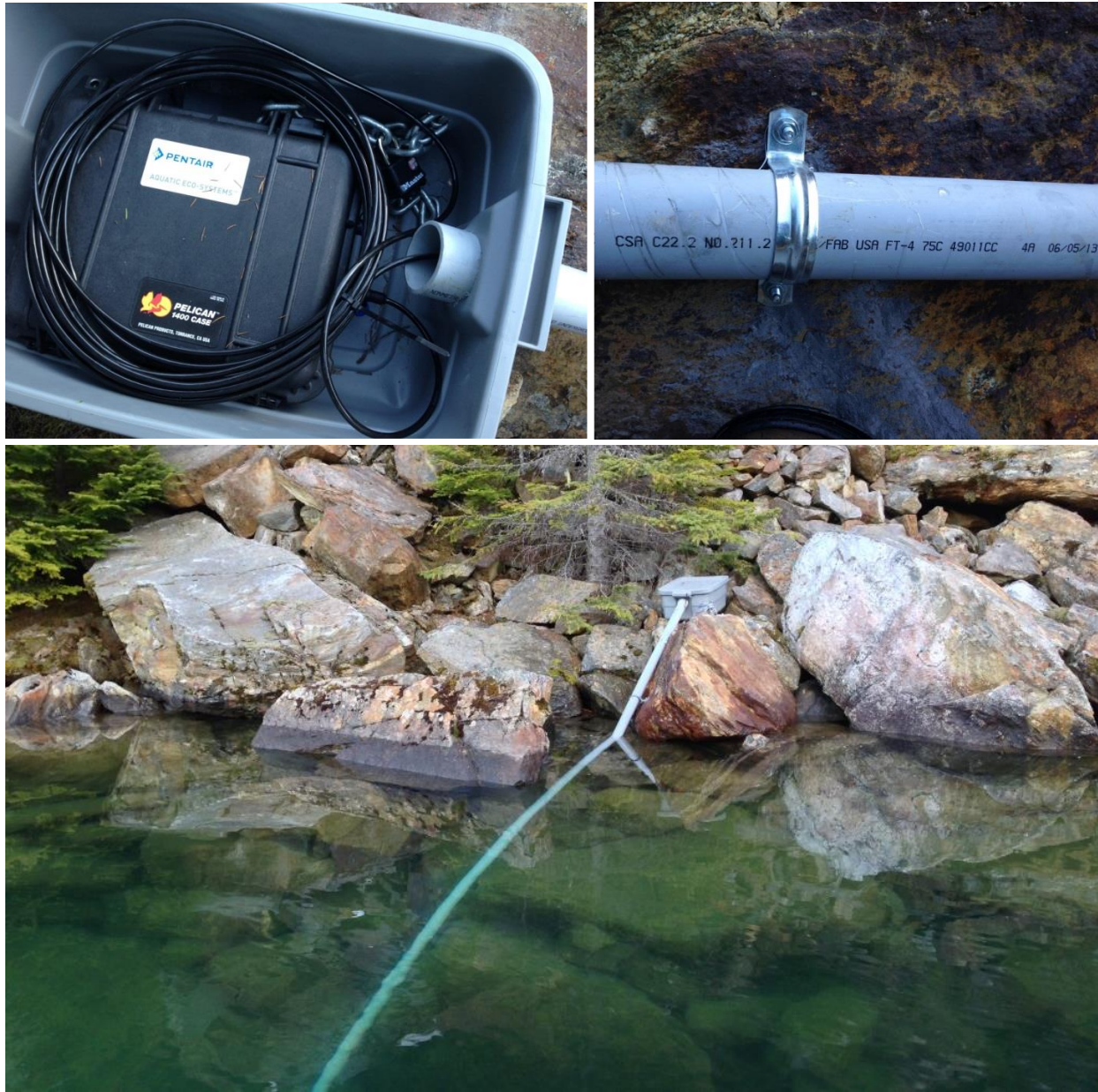
Figure 5. TGP meter deployment totes, anchoring detail and pipe set-up.
