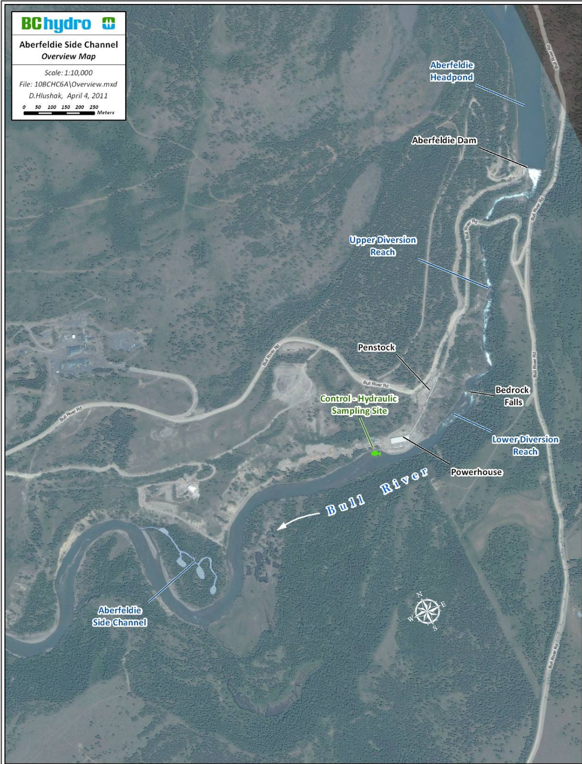
Figure 2 Layout of the Aberfeldie hydroelectric generating facility, diversion reach and side channel compensation habitat.
