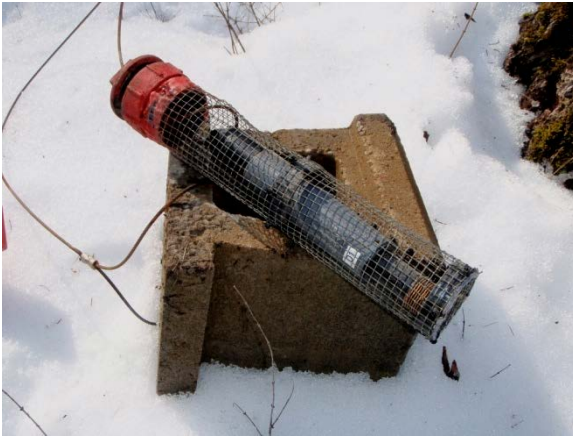
Figure 4 HOBO U-26 dissolved oxygen logger in protective wire mesh tube secured to anchor.
