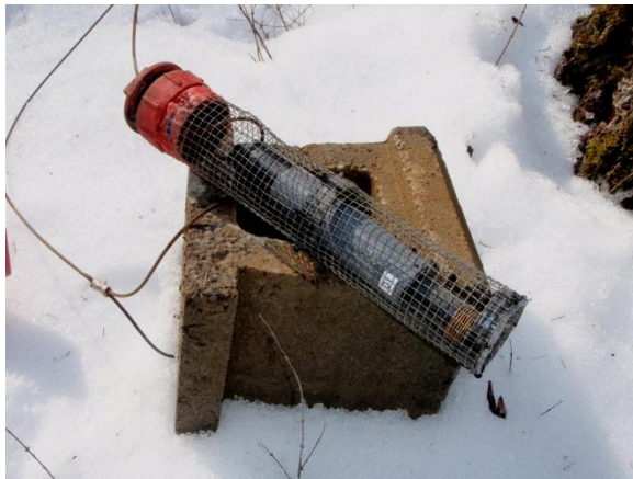
Figure 3 HOBOT U-26 dissolved oxygen logger in protective wire mesh tube secured to anchor.
