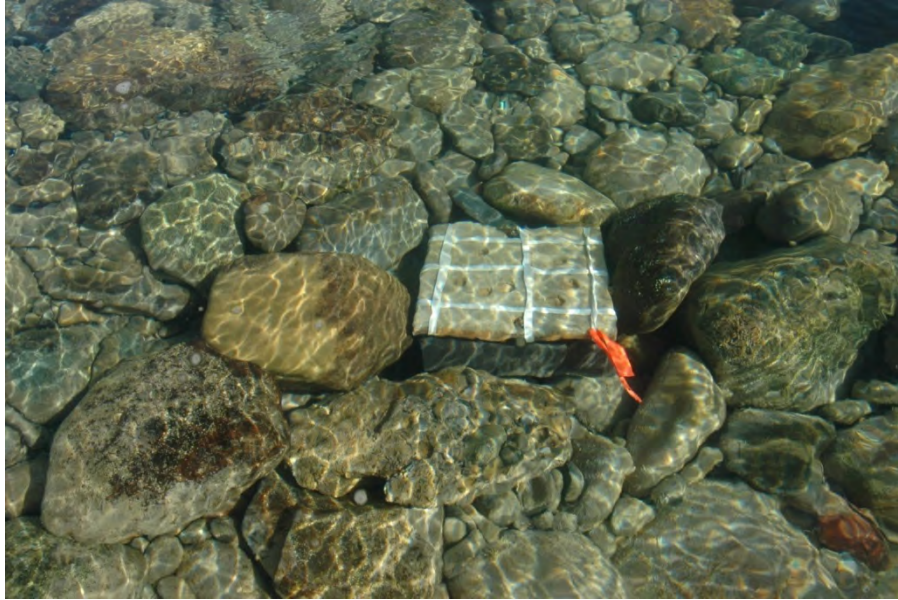
Figure 6. Image of a periphyton plate installed in the Bull River.
