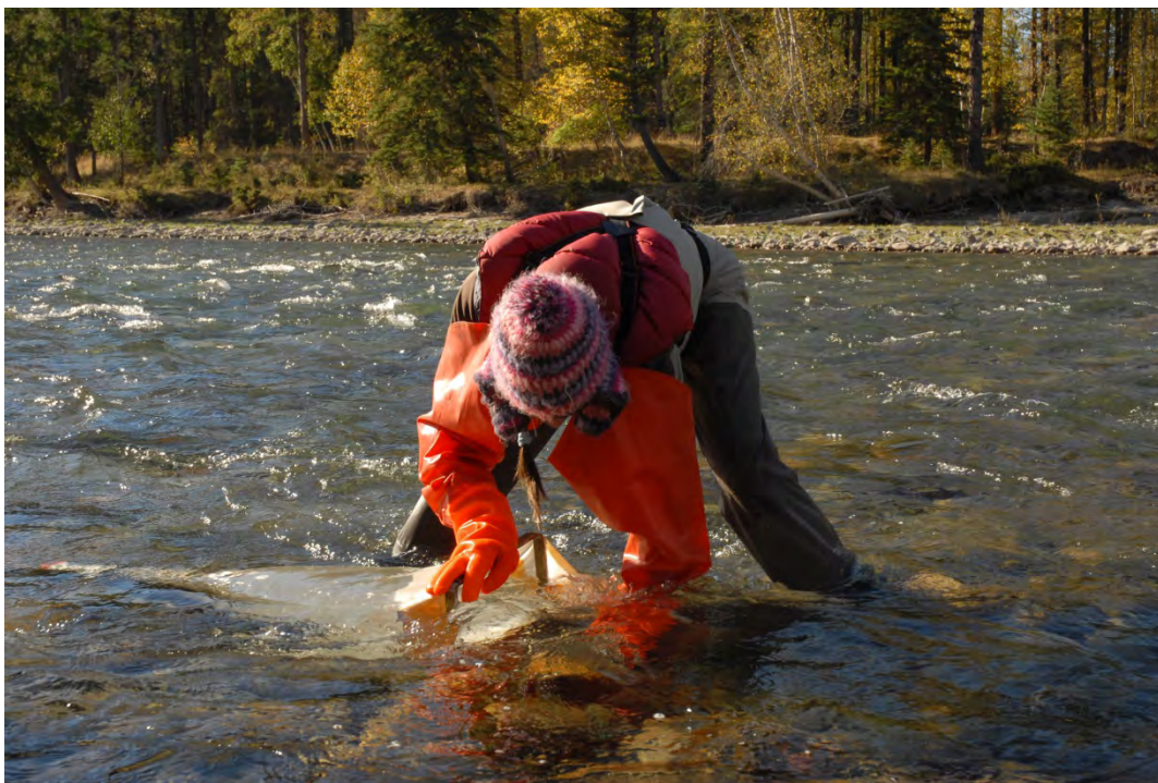
Figure 7. Image of Surber net being used for collection of benthic invertebrates in the Bull River.
