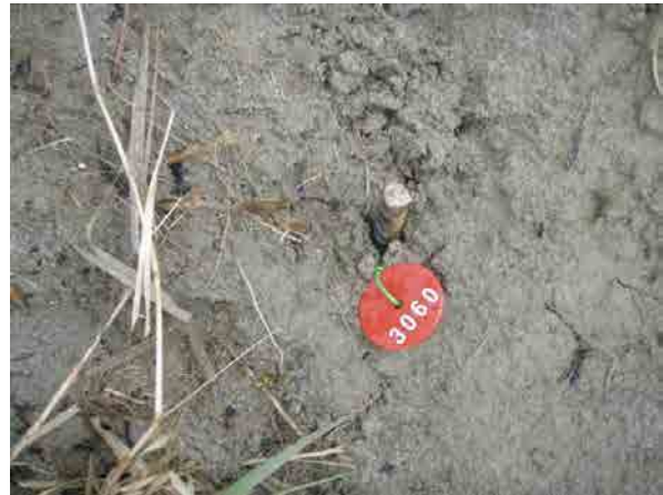
Photo 3.4: Erosion Monitoring Pin (Installed)
