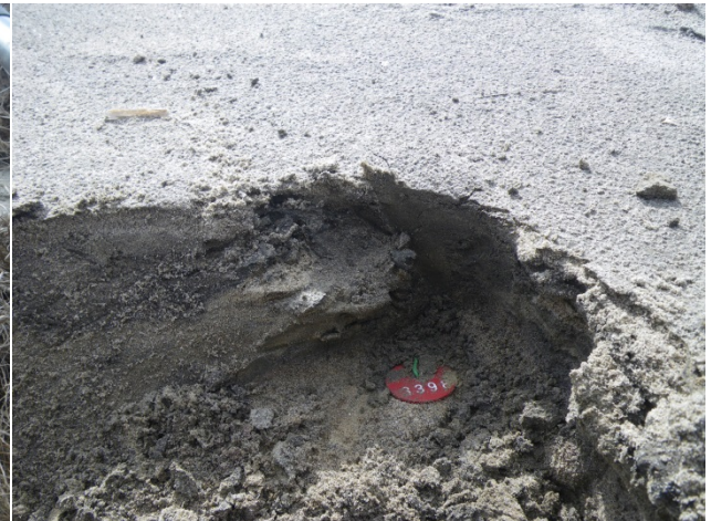
Photo 4-2: Erosion Pin Covered by Deposition of Sediment (April 2012).
