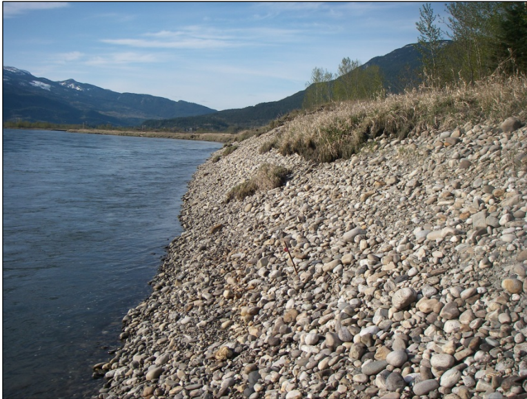
Photo 13: Site B Control, Grassy Blocks Migrating Down Mid Bank Slope, Erosion Pin in Foreground (April 20, 2015)
