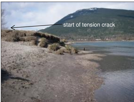
Photos 4-16 & 17: Site A2 Downstream Control, tension crack behind top of bank. (April 23, 2013)
