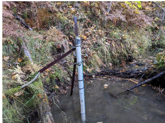
Photo 40: Burton Creek Gauge Following Re-Securing During Fall Visit (October 17, 2024)
