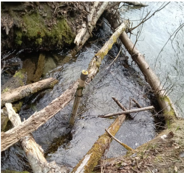
Photo 1: 2024-04-17 Gauge attached to rotting log
