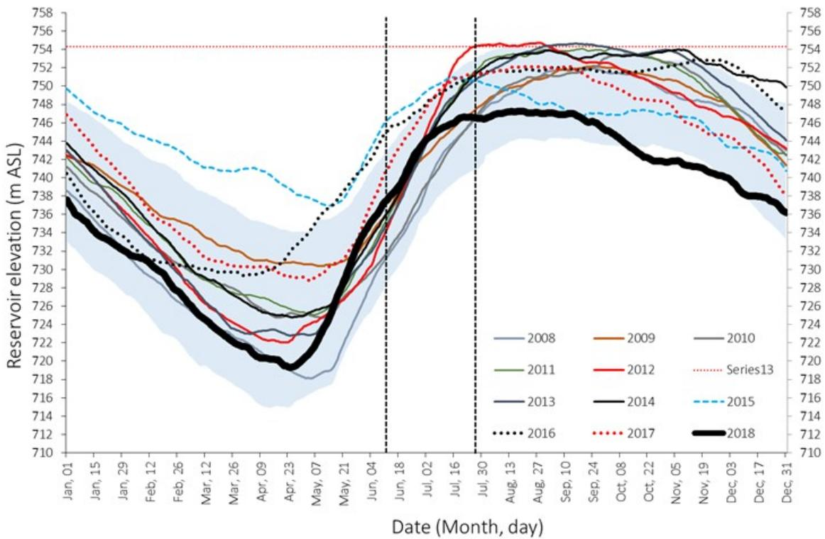
Figure 4-1: Kinbasket Reservoir elevations (m ASL) in 2007, 2008, 2010, 2012, 2014, 2016 and to October 10, 2018. The shaded area indicates the 10<sup>th</sup> and 90<sup>th</sup> percentile (1976 to 2018). The 754 m and 741 m ASL elevations are indicated (red dashed horizontal line). Vertical black dashed lines represented the min and max date of sampling (all years).
