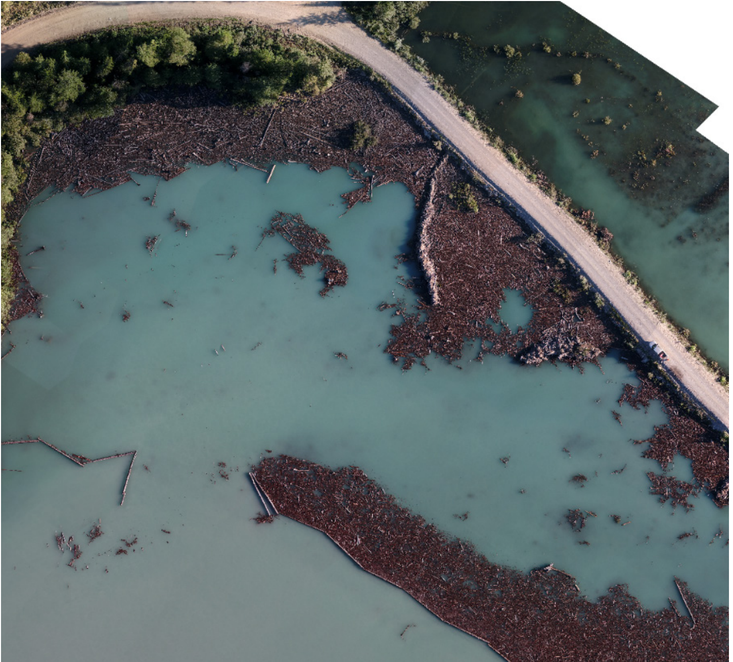
Aerial image of the log-boom breach at Bush Arm following a windstorm in August 2020. Image obtained by Murray Chapple, Sterling Lumber Co Ltd.
