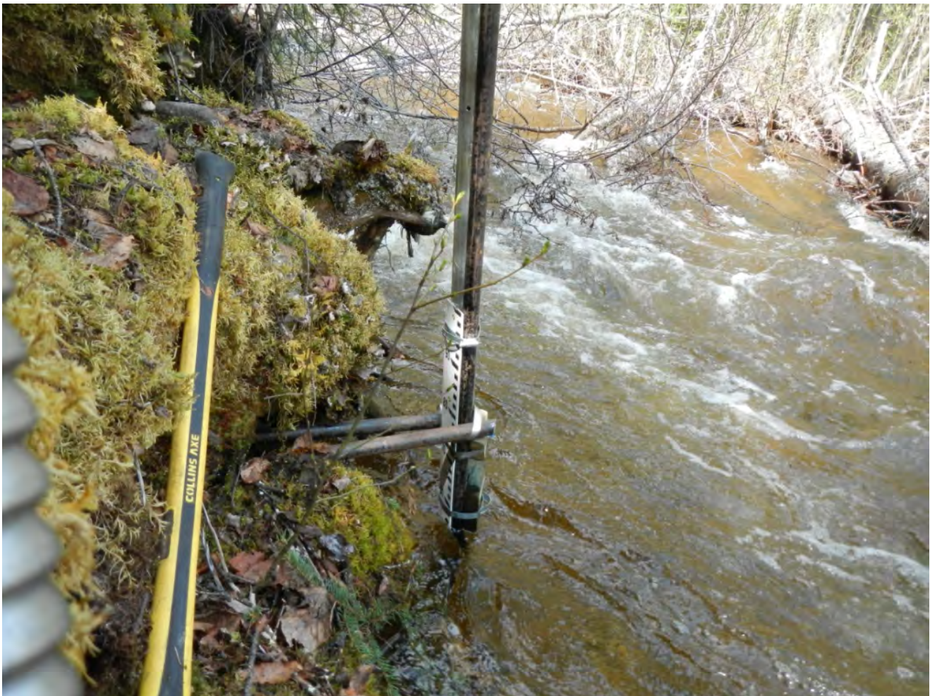
Photo 2. Housing for water level and temperature probe at Ole Creek gauging station.
