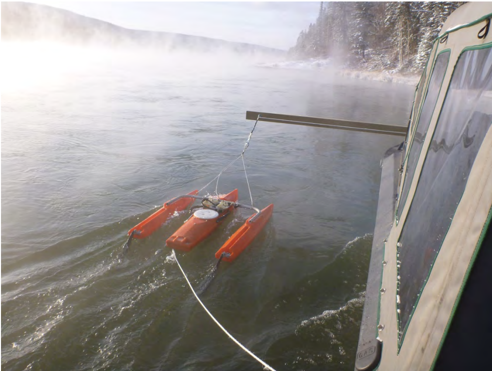
Photo 2 Discharge measurement with ADCP alongside jet boat
