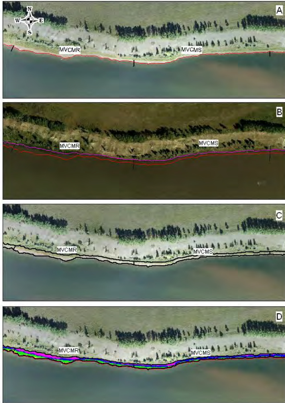
Figure 2.1 Illustration of habitat type mapping steps. A -- The upst. and dwst. boundary of each habitat unit was delineated on the minimum discharge (283 cms) orthophoto base map. B -- The upst. and dwst. boundary of each habitat unit was set perpendicular to the channel margin and then extended to the maximum extent of the wetted surface area, which was represented by the maximum discharge (1,982 cms) orthophoto base map. C -- The maximum surface area of the habitat unit was delineated by forming a polygon around the perimeter of the unit. The unit boundary was juxtapositioned with the adjacent habitat unit boundaries to eliminate overlap. D - The total wetted surface at each of the five discharges was overlain with the habitat unit polygon to generate a wetted surface polygon specific to that habitat unit.
