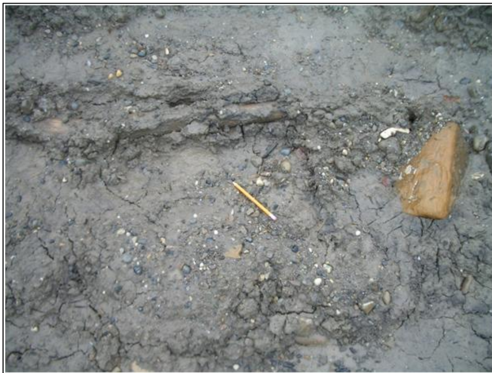
Photo 10: Taken on 5-19-2009 at Existing Dunlevy Site (In-situ native clayey silt found in parts of the bank at Dunlevy and was present in the vicinity of the areas most subject to slumping).
