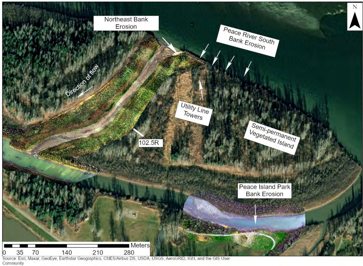
Figure 2.2 Satellite image of 102.5R side channel, overlaid with 2019 drone photos, illustrating areas of erosion that were specifically inspected.
