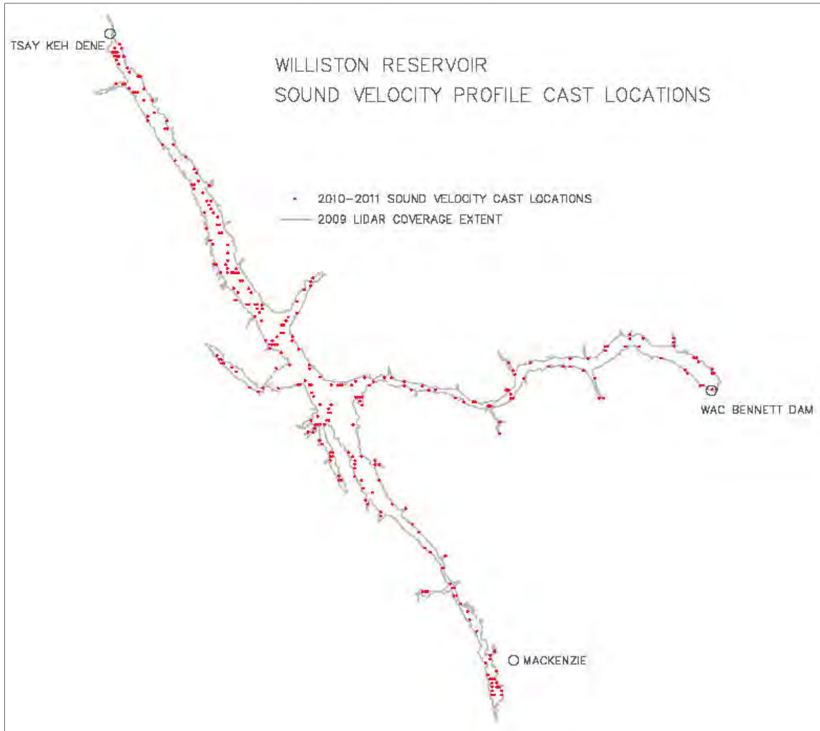
Figure 20 - Distribution of the 2010-2011 sound velocity casts.
