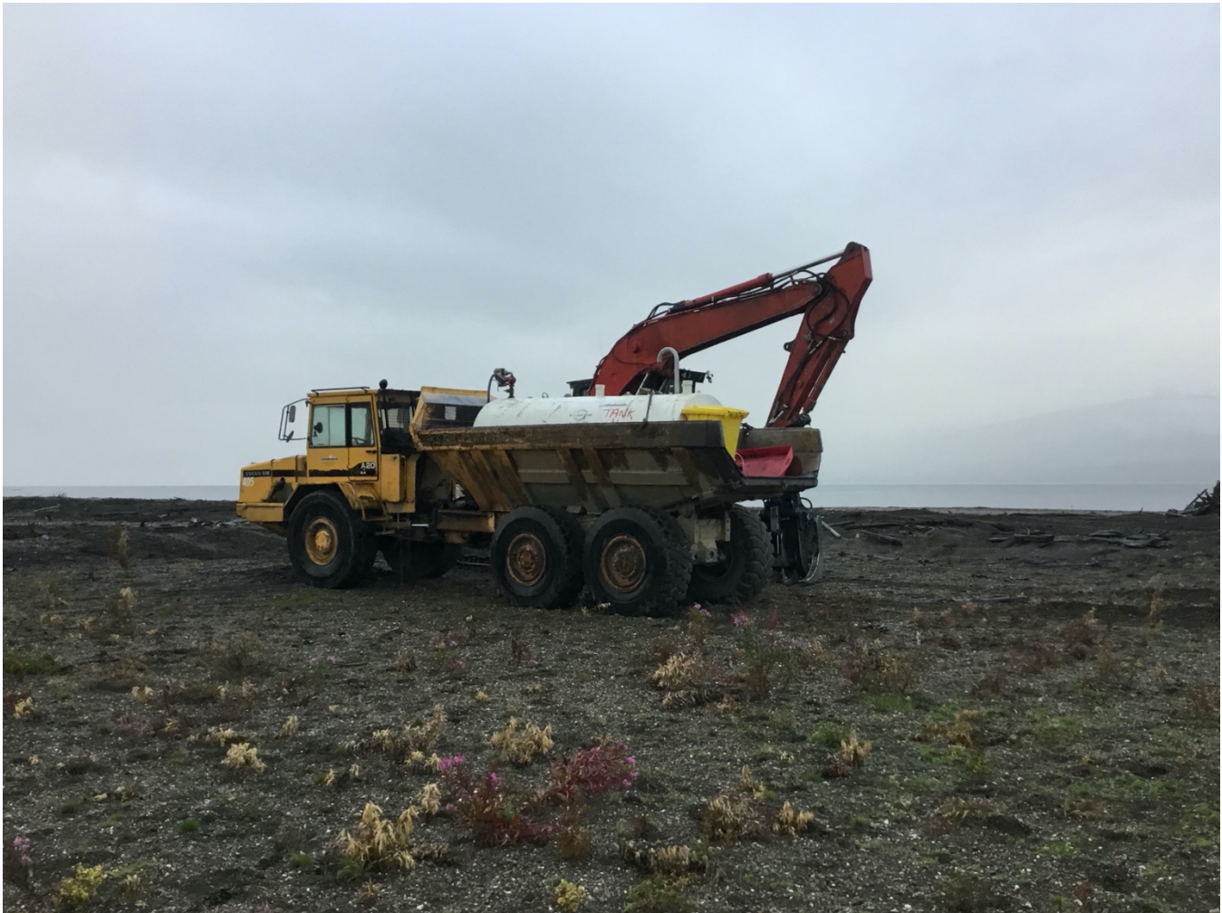
Figure 14: Fuel bowser with large spill kit.
