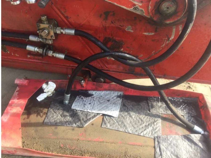
Figure 28 : Managing and replacing leaking hoses with spill kit and tray.
