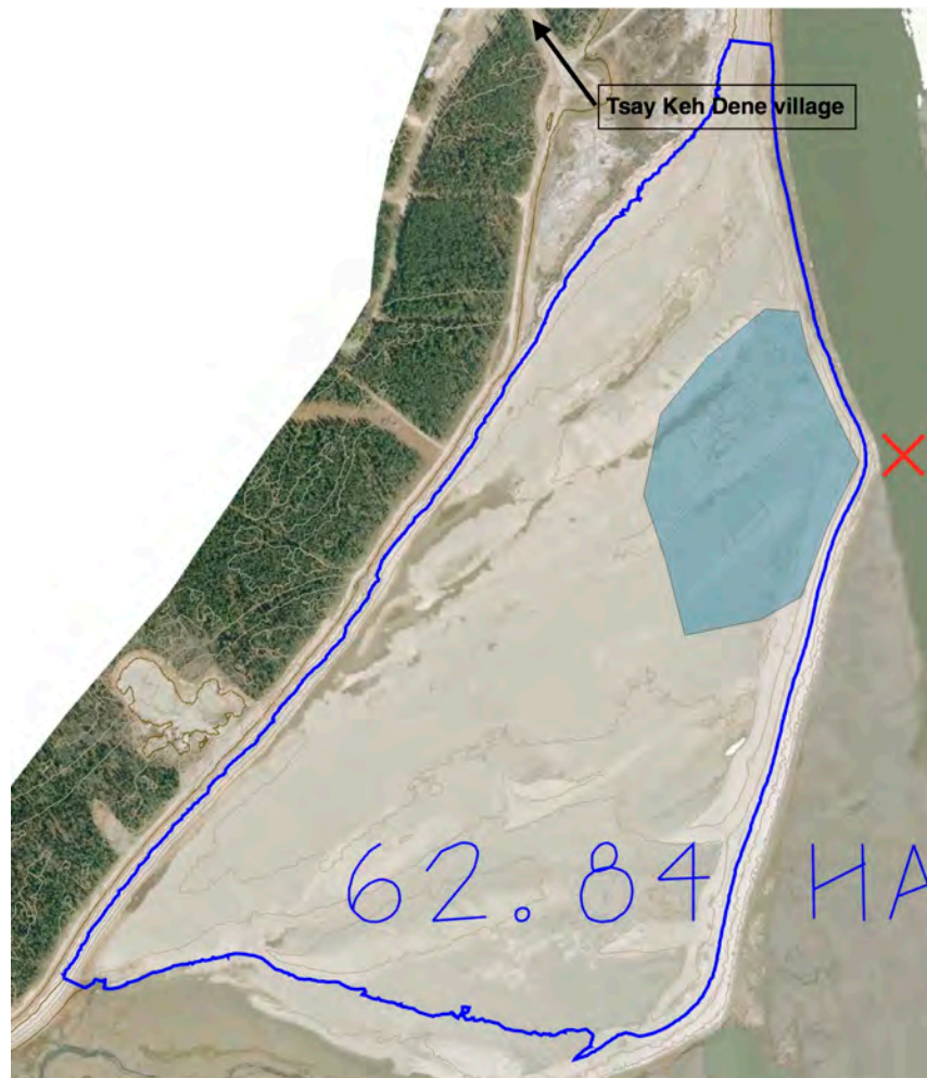
Figure 2: Proposed location of water intake and the presumed wetted zone. We will move the pumps and sprinklers in response to rising reservoir levels to ensure we are always maximizing our wetted area.
