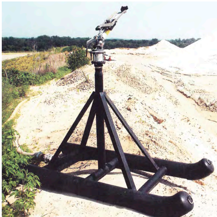
Figure 1: Water tank skid for mounting and transporting the Big Gun
