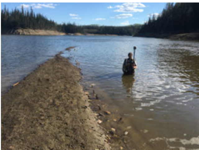
PHOTO 9: Survey of Toe of Berm 'G' on Creek Side
