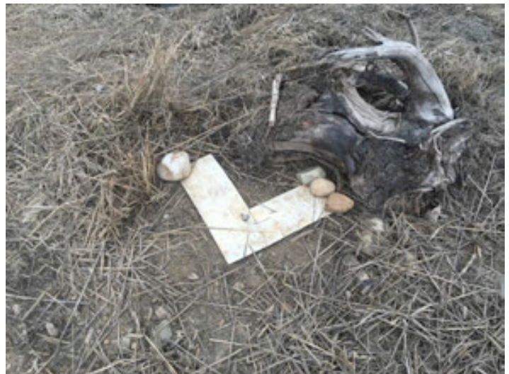
PHOTO 37: UAV Marker (surveyed)
