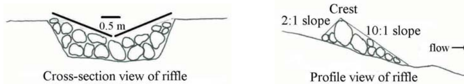
Figure 24. Conceptual design for riffles. Dimensions are from Newbury and Gaboury (1993).
