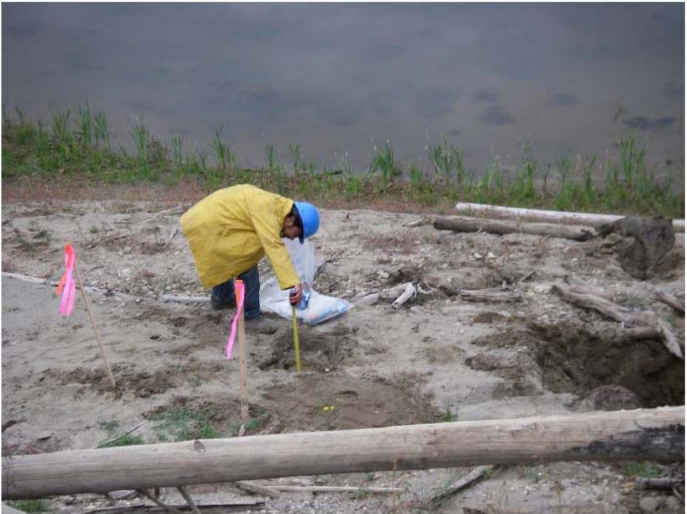
Photo 3: Conducting a percolation test at Site 6-2
