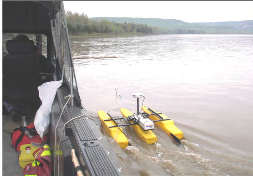
PHOTO 10 – Sontek RiverSurveyor S5 Acoustic Doppler Current Profiler attached to a boom and held off the bow of the jet boat.
