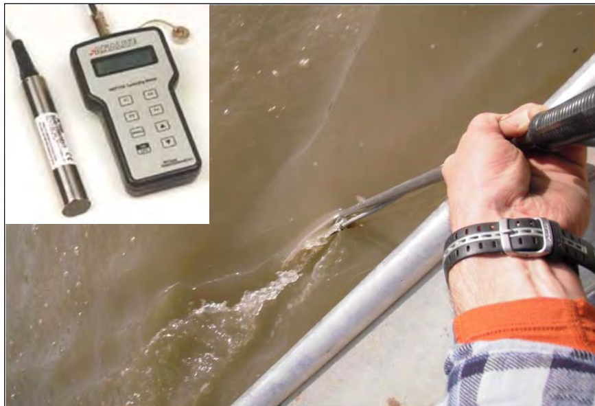
PHOTO 11 – Analite NEP 160 turbidity sensor attached to a 1 m rod and held 20 cm below the water surface from the side of the jet boat.
