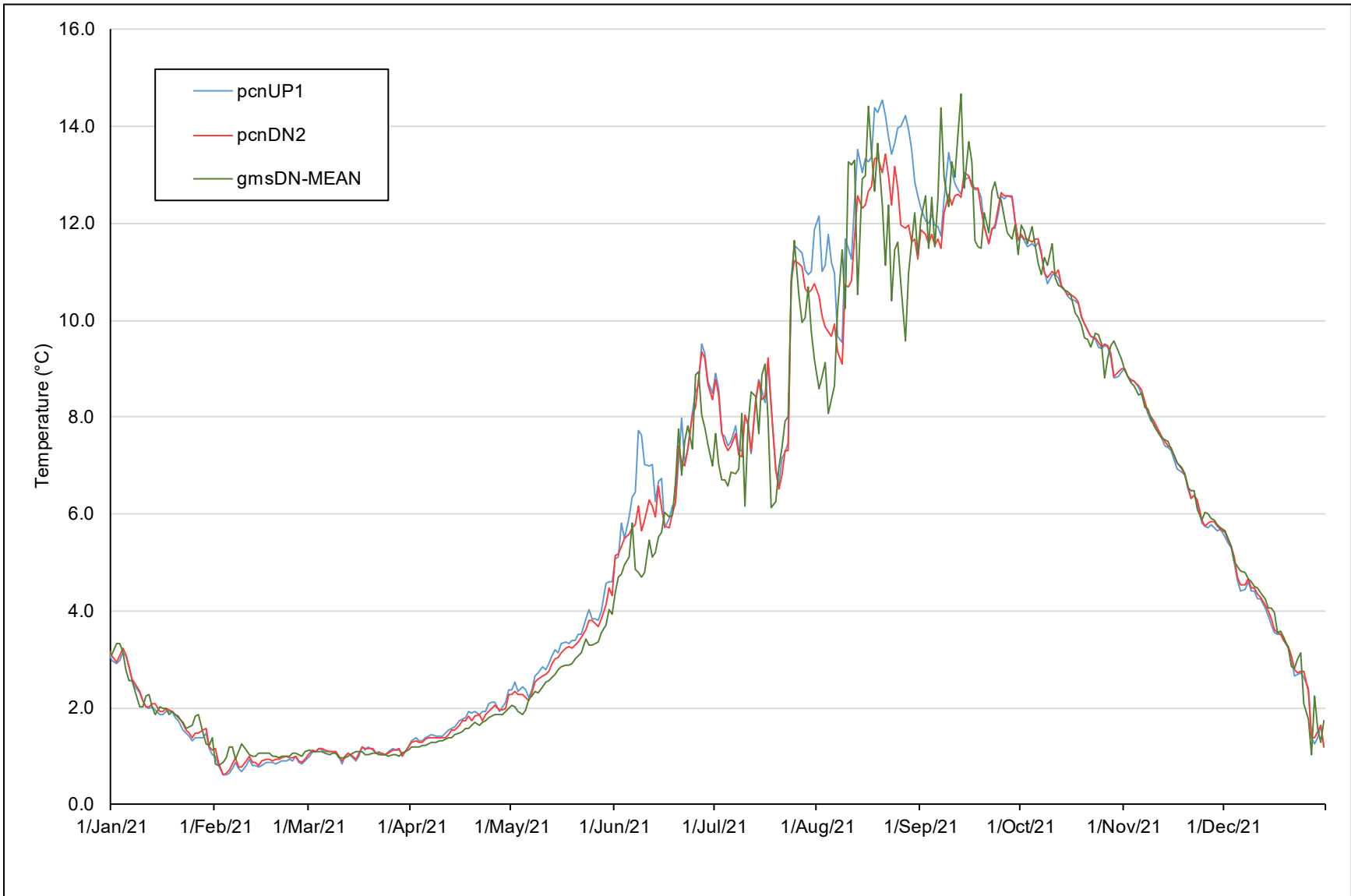
Figure 4. Comparison of daily mean water temperature at Peace Canyon forebay surface (pcnUP1), Peace Canyon tailrace (pcnDN2), and WAC Bennett Dam tailrace (gmsDN-MEAN) during Year 11, January 01, 2021 – December 31, 2021.
