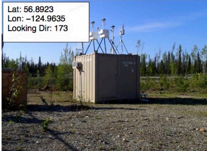
Figure 13: Tsay Keh Dene Regional Monitoring Network and Reference Station – E-Sampler is on top of enclosure.
