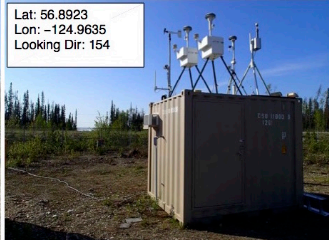
Figure 13: Tsay Keh Dene Regional Monitoring Network and Reference Station – E-Sampler is on top of enclosure.
