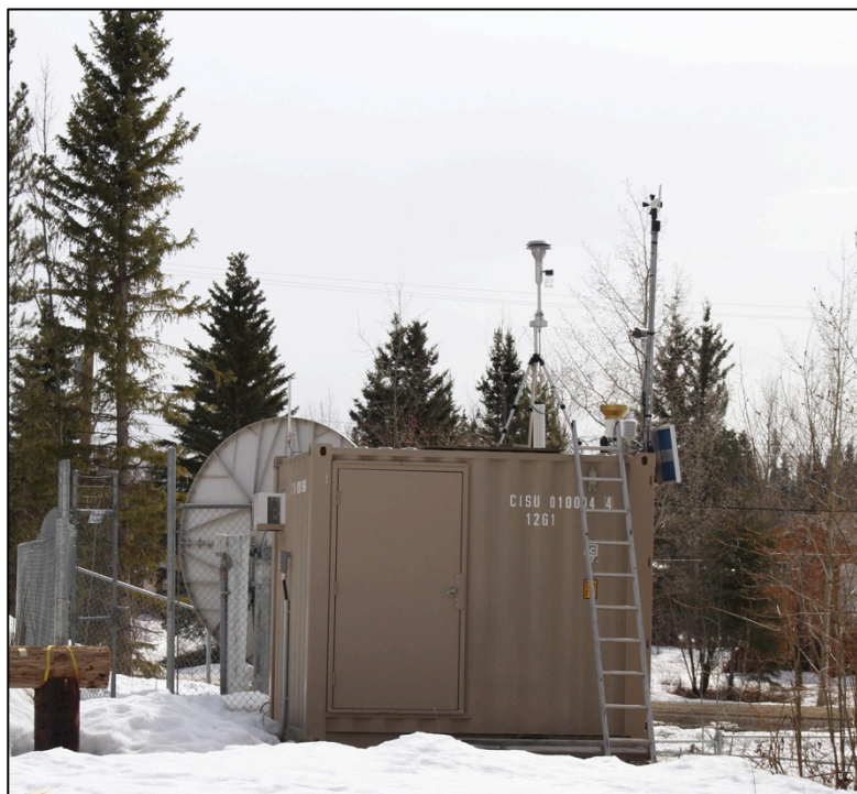
Figure 27: Kwadacha Air Quality Monitoring Station
