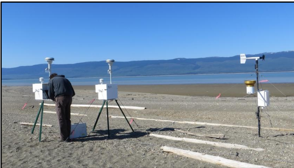
FIGURE 2.7. DEPLOYMENT OF THE BGI PQ200 PM 10 AND PM 2.5 SAMPLERS AND ASSOCIATED METEOROLOGICAL INSTRUMENTATION AT CHOWIKA BEACH.
