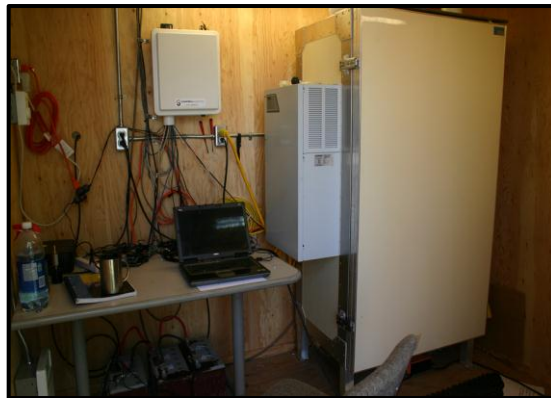
FIGURE 2.2. THE INTERIOR OF THE ENVIRONMENTAL ENCLOSURE SHOWING THE TEOM, DATALOGGING INSTRUMENTS, AND NETWORKING HARDWARE, TSAY KEH.
