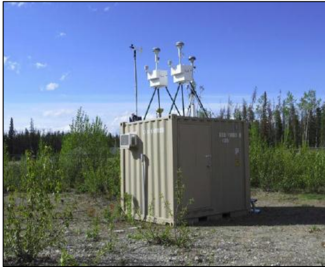
FIGURE 2.1. THE STEEL BUILDING IN TSAY KEH THAT HOUSES THE TEOM, DATALOGGING INSTRUMENTS AND PROVIDES A PLATFORM FOR THE METEOROLOGICAL SENSORS AND THE TEOM INLET.
